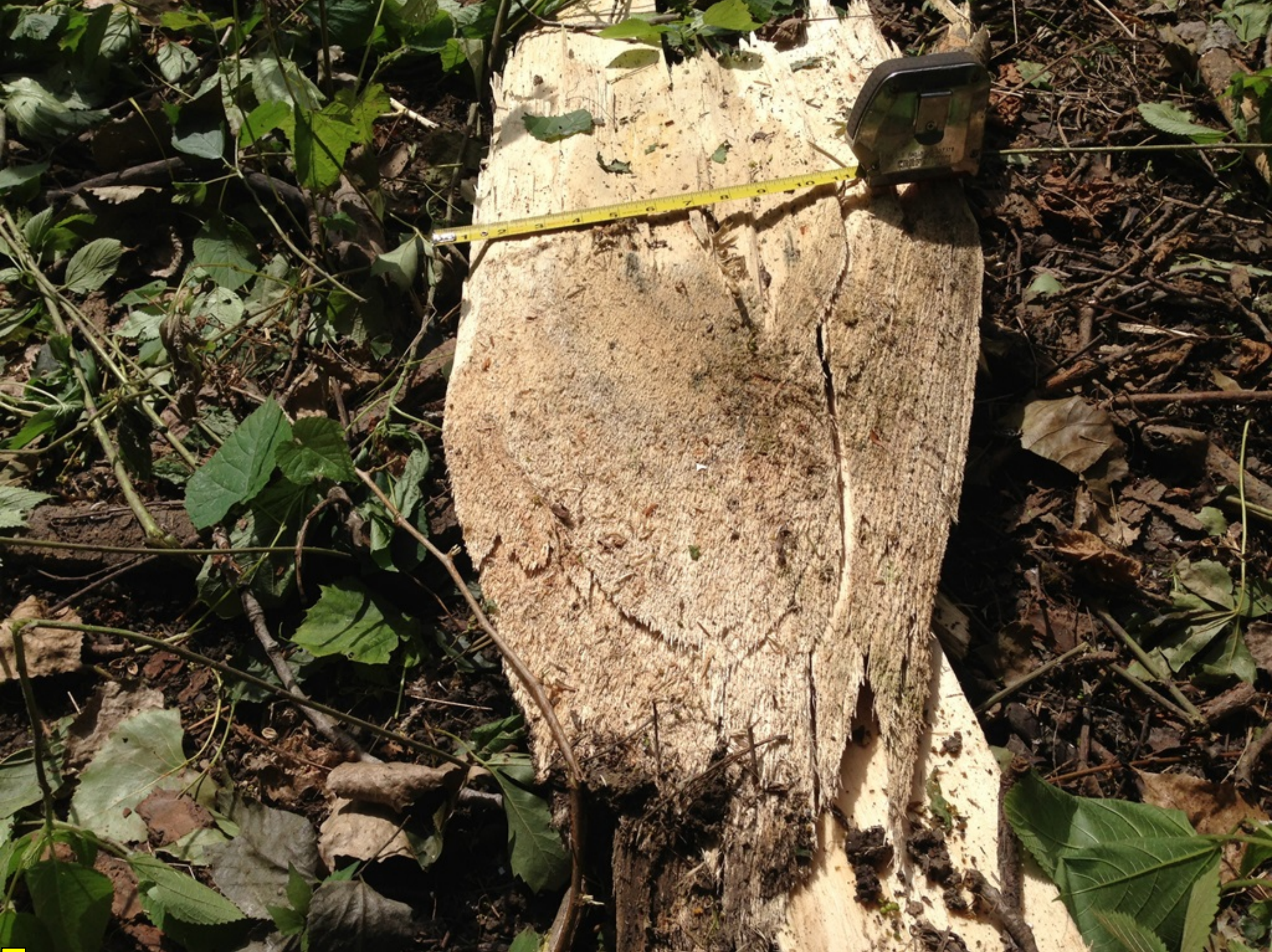
Photo 8. Piece of wood with a 13 X 18 inch slash and paint transfer found at the base of the tree.
