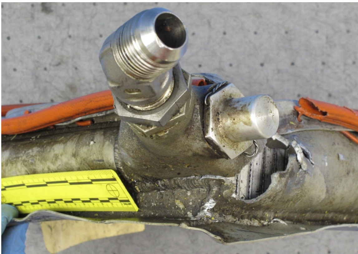
Figure 5 – The fractured plenum, rotated 45° from Figure 4, showing the crack along the weld.
