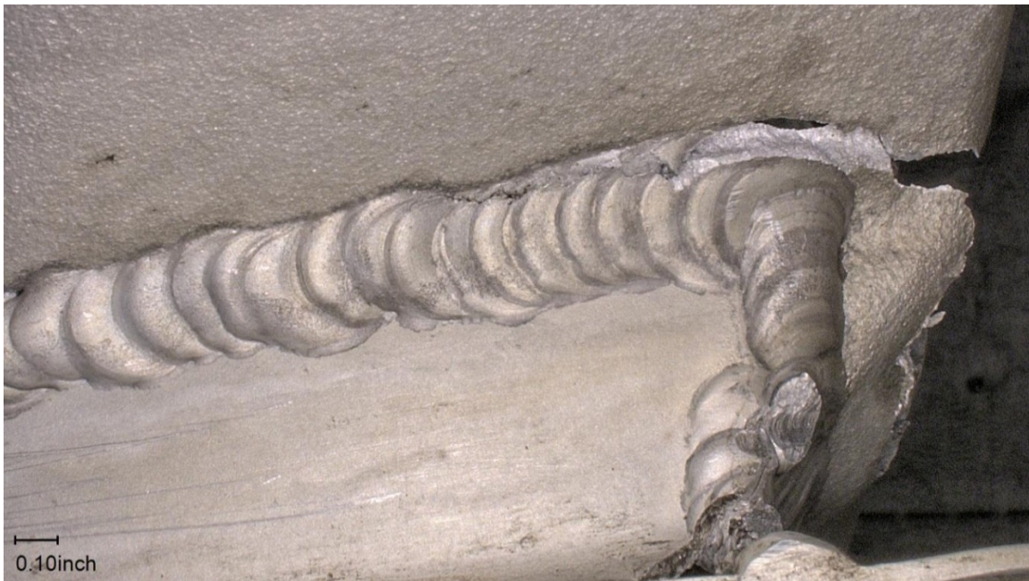
Figure 6 – The cracked weld from Figure 5, after cleaning with ethyl alcohol.
