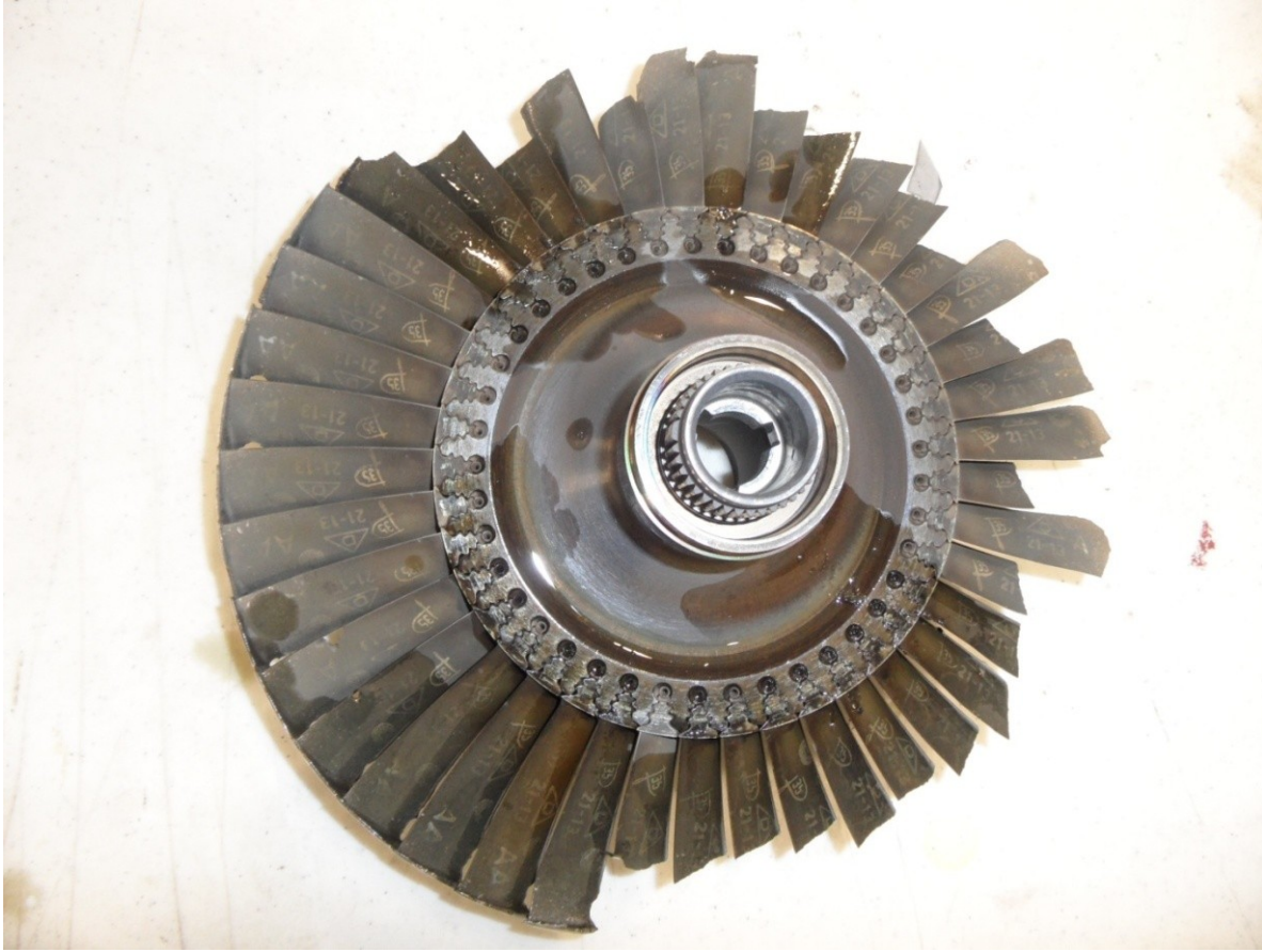
Figure 22. PT disk assembly showing severely localized blade loss
