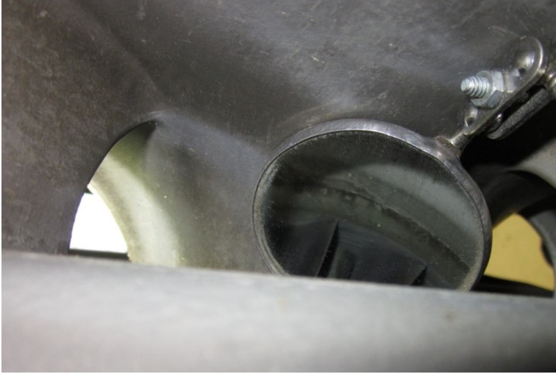
Figure 14. 1 st stage of compressor viewed through the engine inlet
