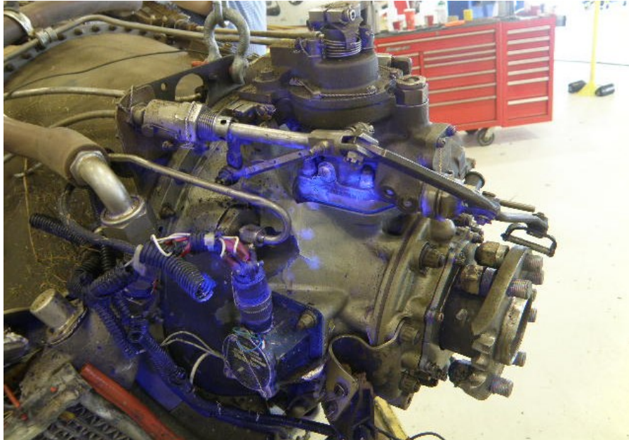
Figure 8. Oil residue fluorescing under UV light
