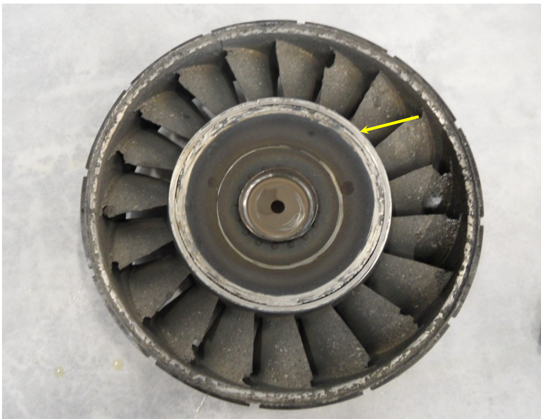
Figure 20. Power turbine vane assembly downstream side showing heavy scoring along the baffle face
