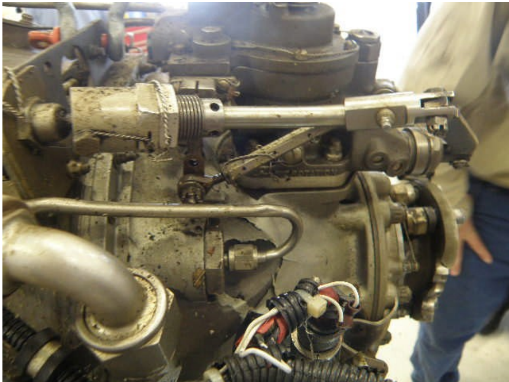
Figure 12. Reset arm-to-beta arm rod
