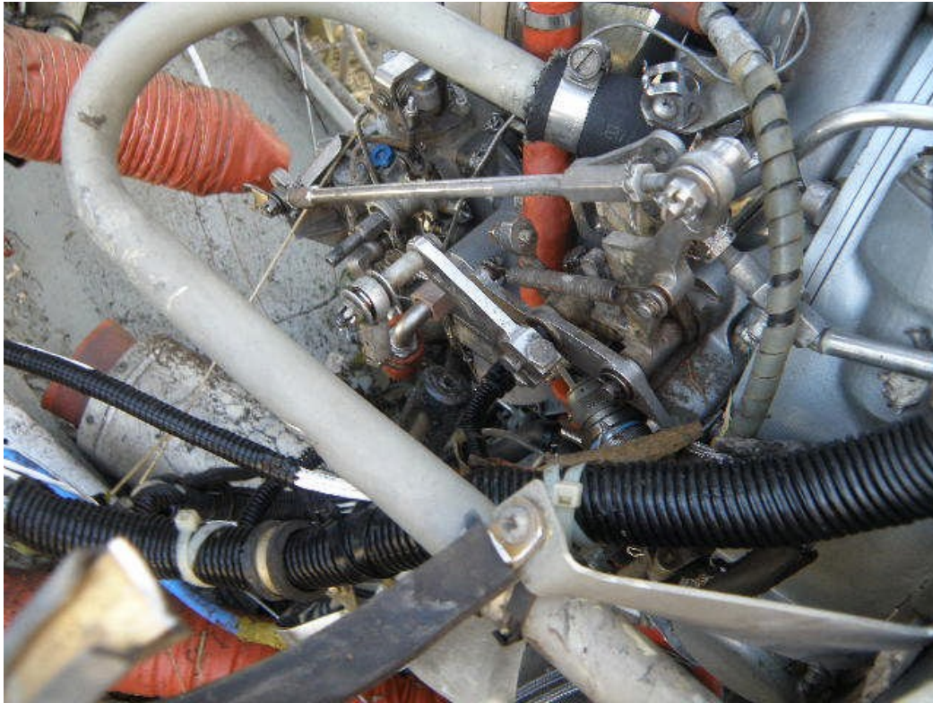
Figure 11. Fuel control unit-to-cambox linkage
