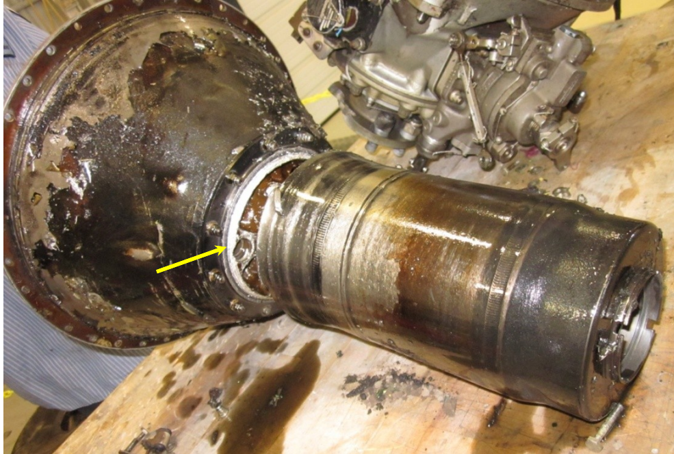
Figure 25. PT shaft housing and rear RGB showing fracture
