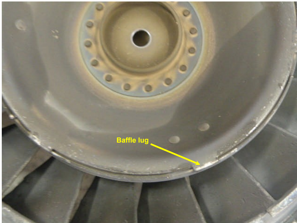
Figure 19. Upstream side of the PT vane assembly showing baffle lug scoring
