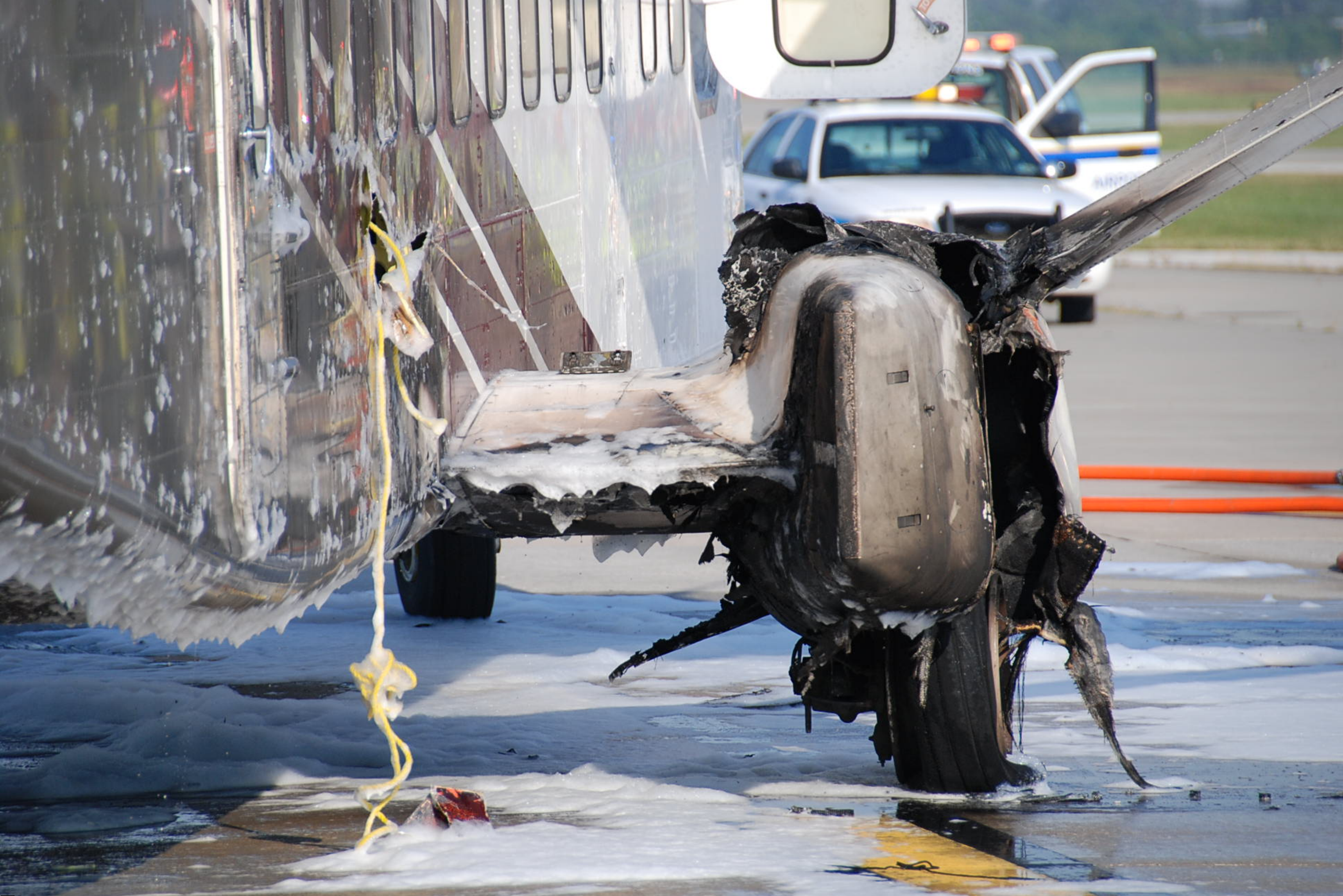
Photo 5 Rear Aspect of Fire Damage to Right Stub Wing Assembly
