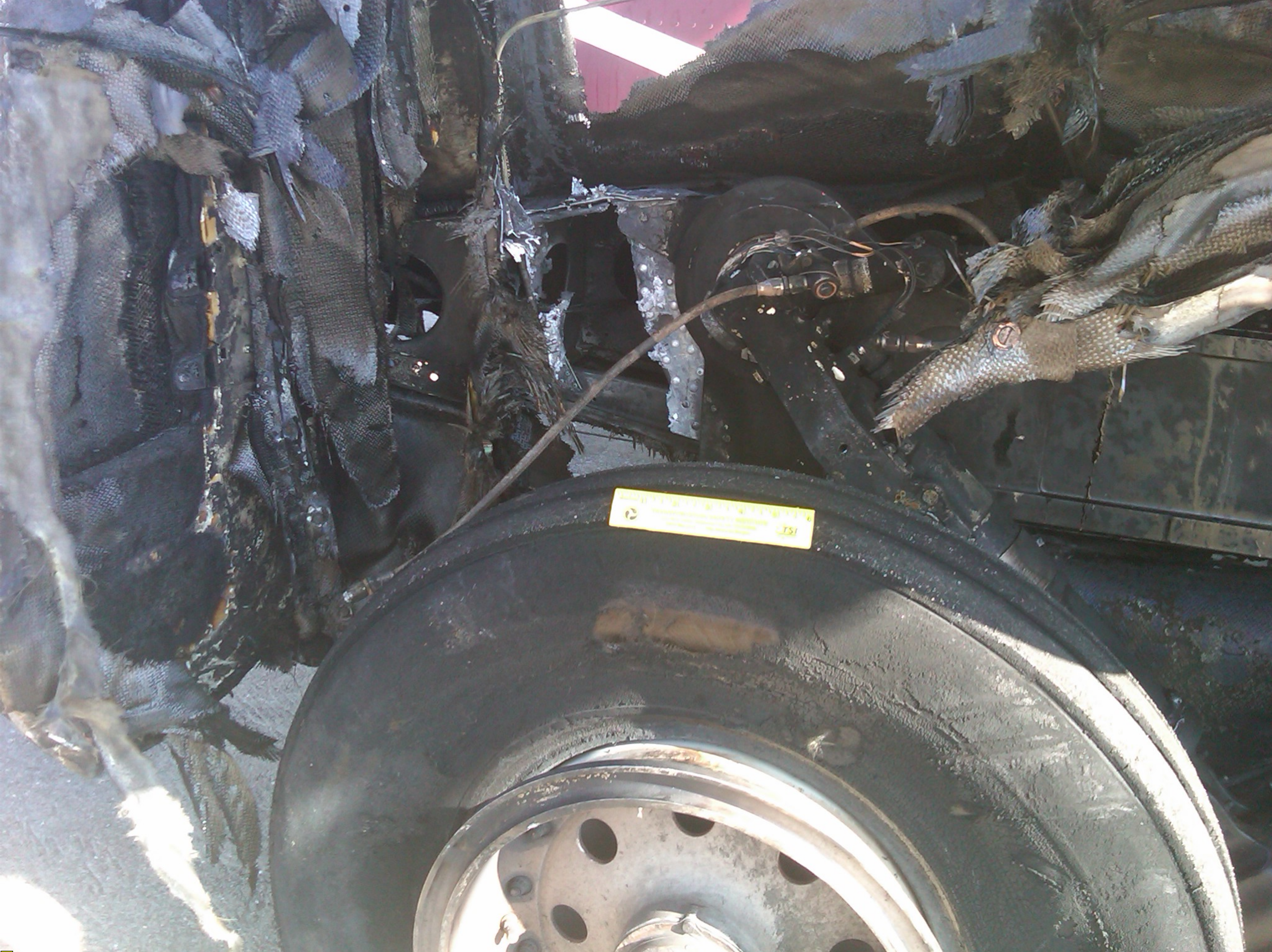
Photo 4 Closeup of Fire Damage to Right Wheel and Brake Assembly
