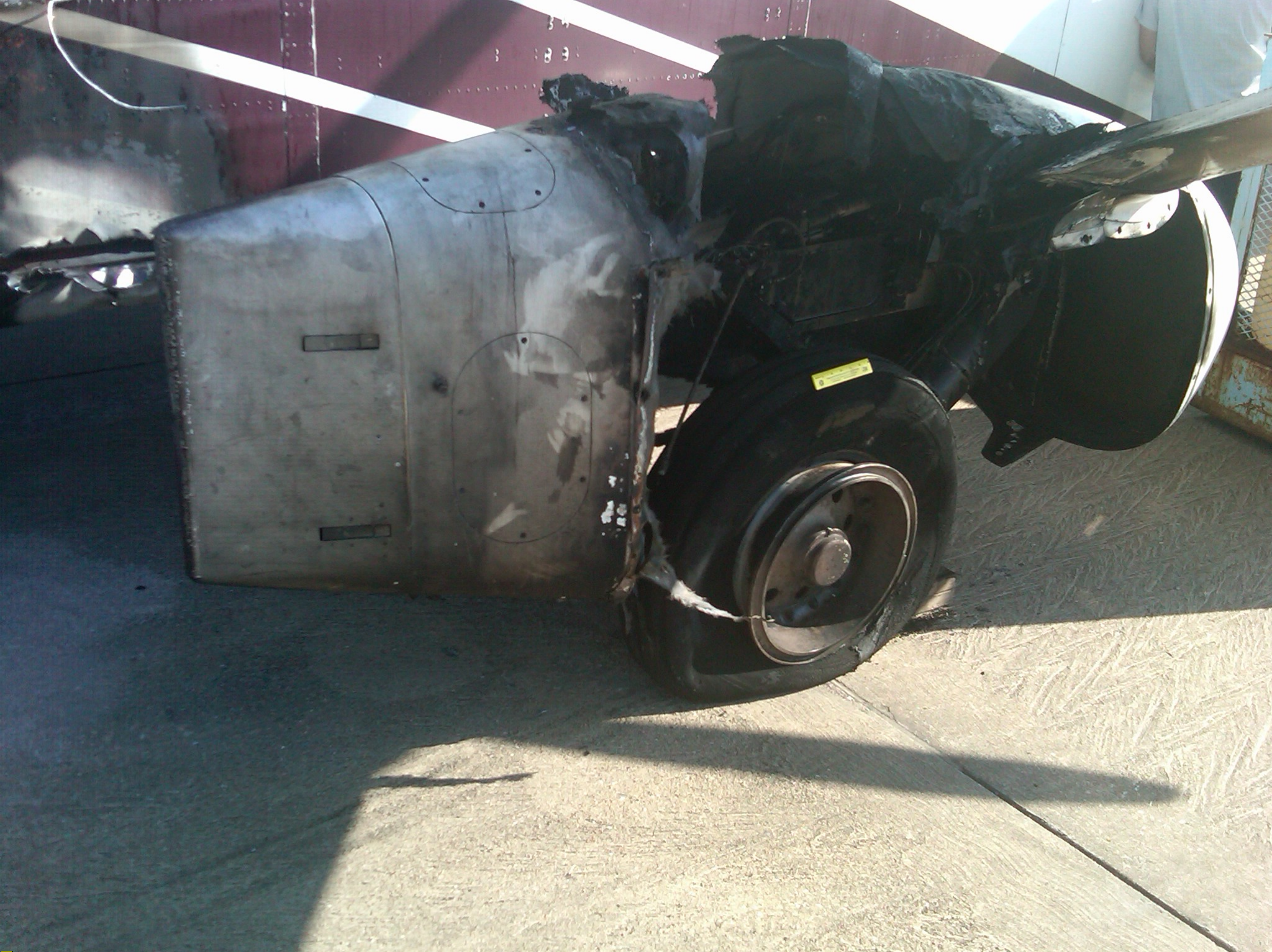
Photo 3 Fire Damage to Right Wheel and Brake Assembly
