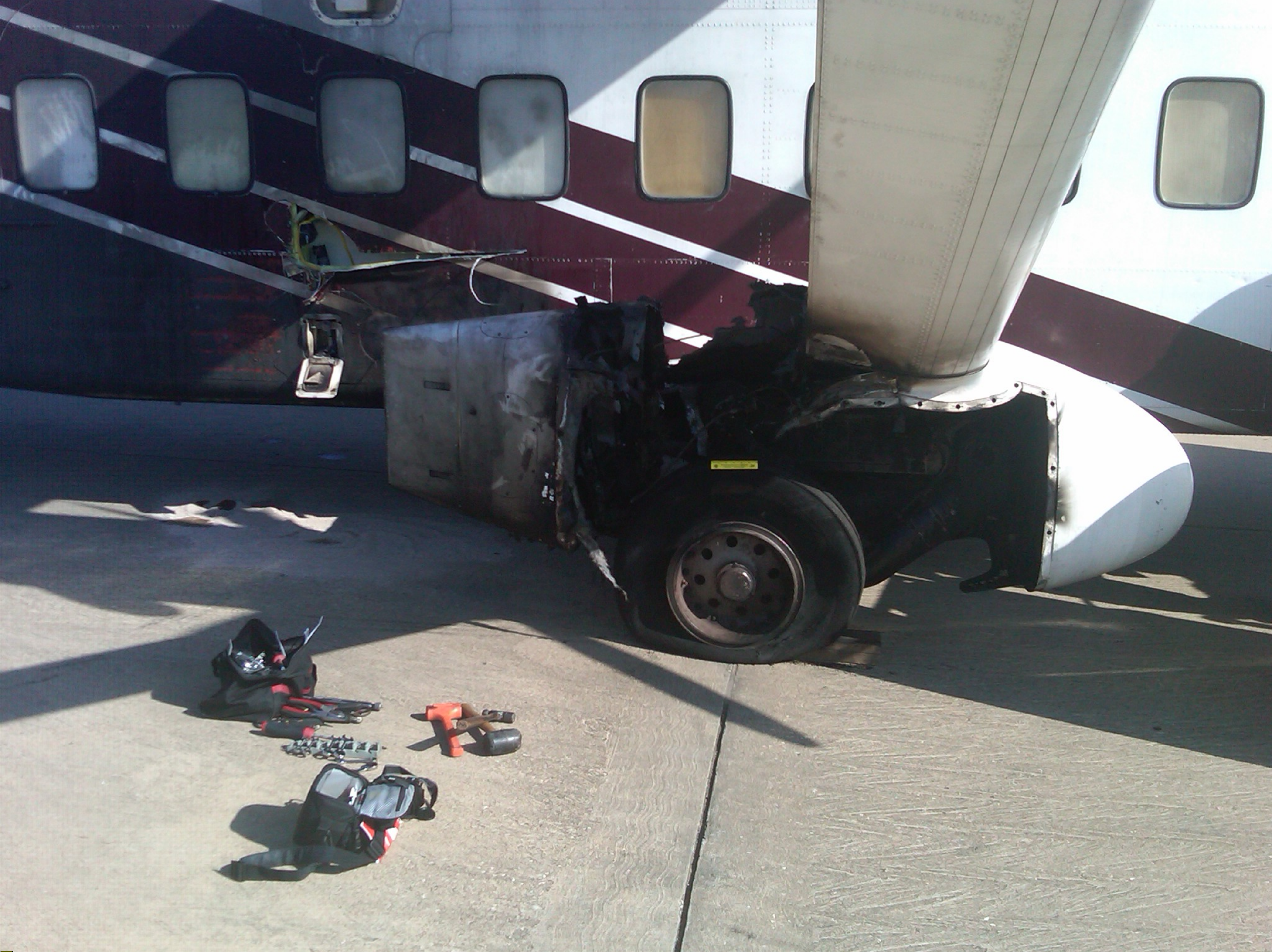
Photo 2 Closeup of Fire Damage to Right Stub Wing Assembly
