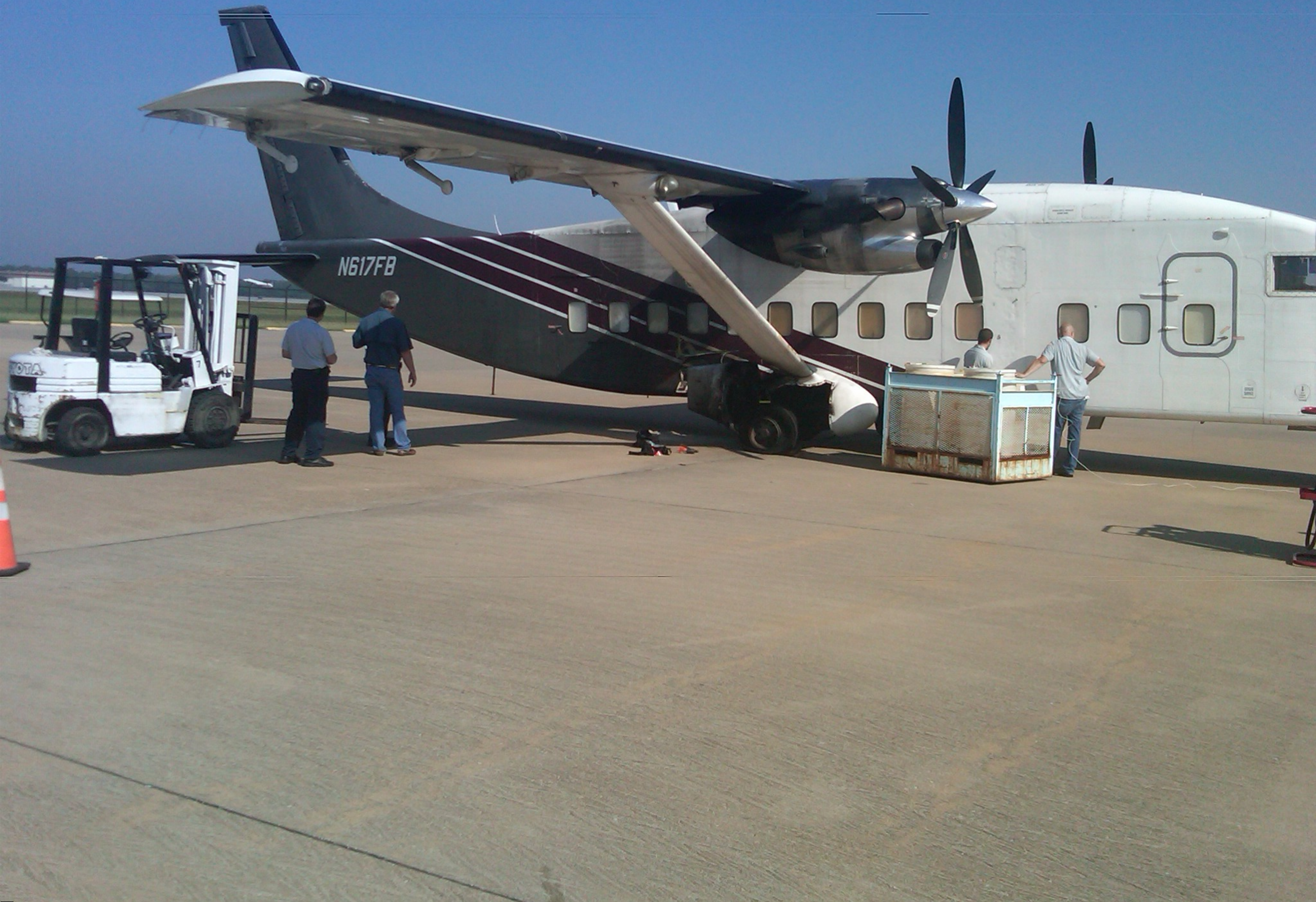
Photo 1 Airplane with Fire Damage to Right Stub Wing Assembly
