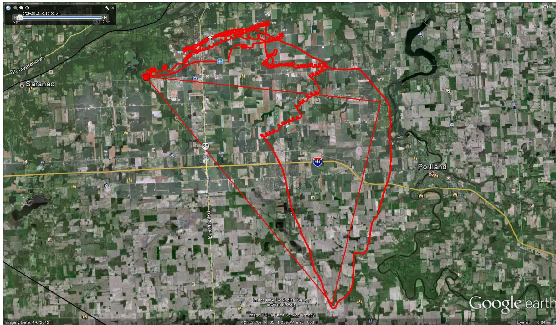
Figure 1. 2-D depiction of the accident flight from Cambridge Aero Instruments IGC data.
