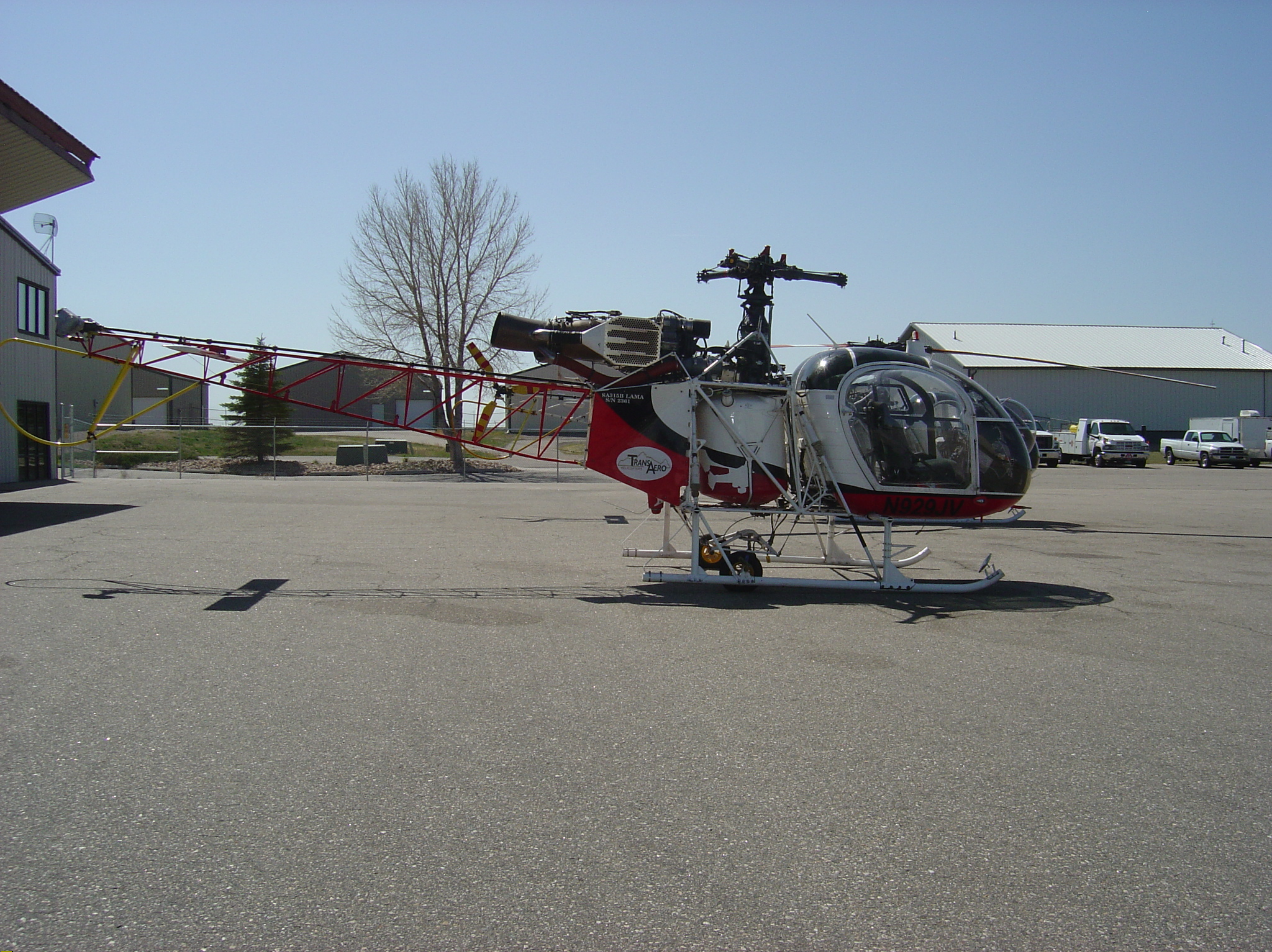
Photo 2 - Right side of helicopter. Tail rotor drive shaft is bent and some hangers are damaged.
