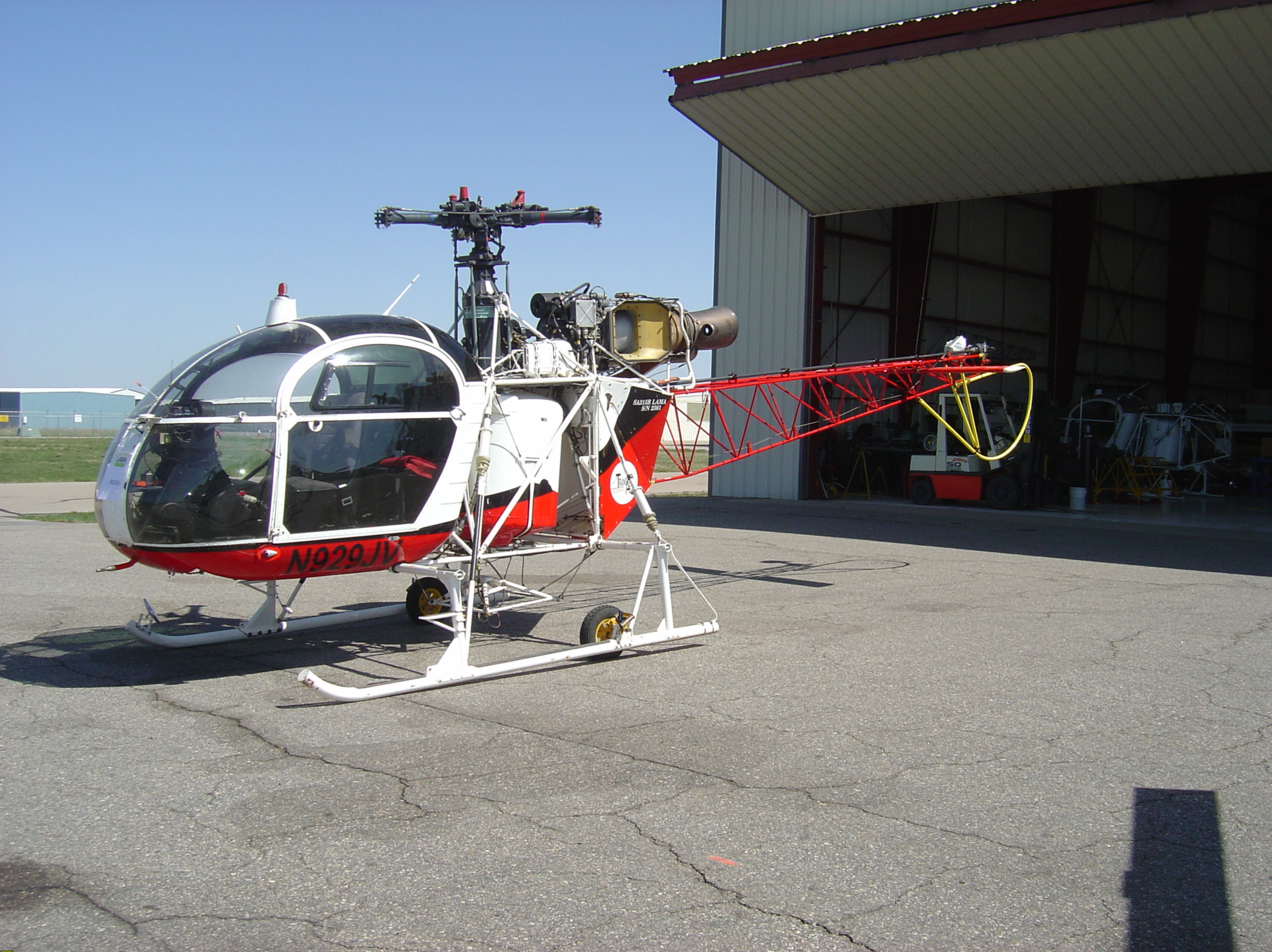
Photo 1 - Left front of helicopter. Main rotor blades have been removed to effect retrieval.
