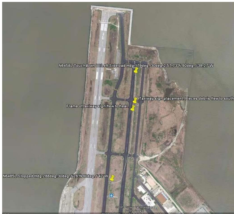
Figure 1 – Showing location of first impacts and the final resting location.
