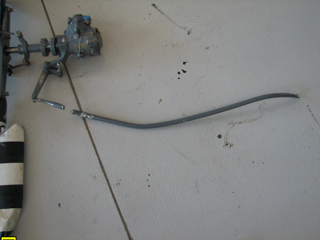
Photo 18. Tail rotor gearbox and broken pitch control tube.
