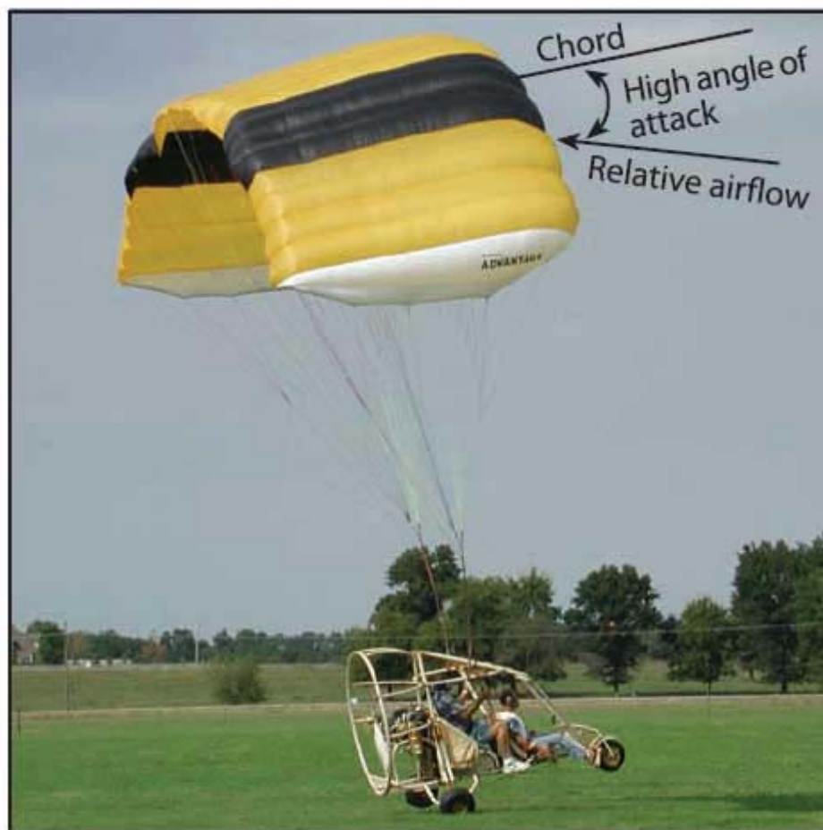
Figure 2-28. Wings stall due to an excessive angle of attack.
