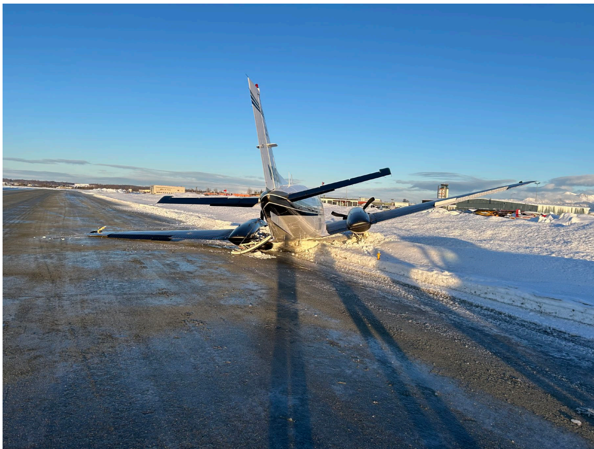
Photograph 2 - Image of accident airplane from behind (Courtesy of airport operations)
