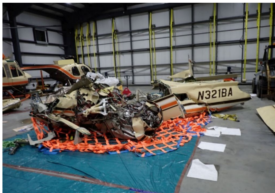
Figure 2 - Fuselage during post-recovery examination (Textron photo)
