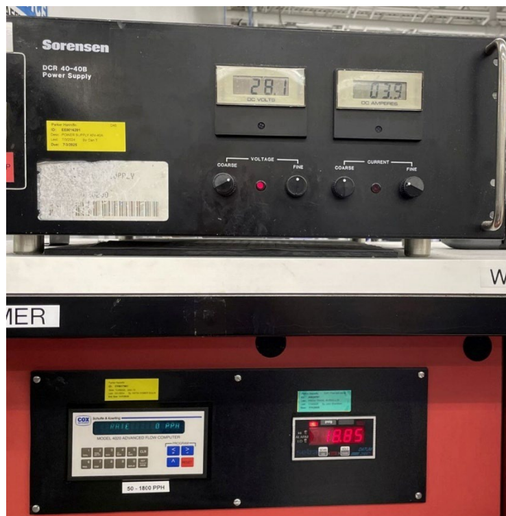
Figure 17 - Test bench readings at 0 pph test point (NTSB photo)
