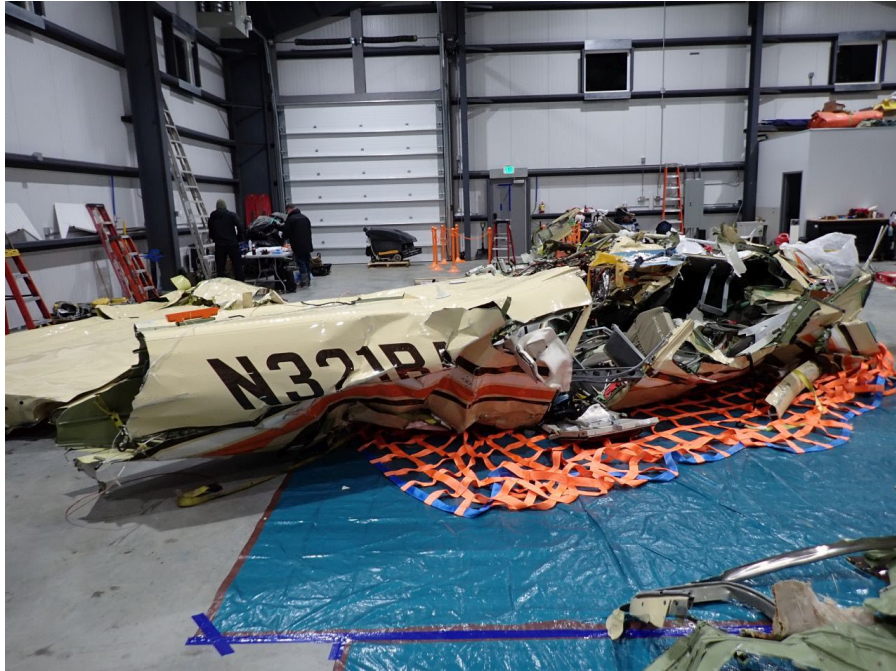
Figure 3 - Fuselage during post-recovery examination (Textron photo)
