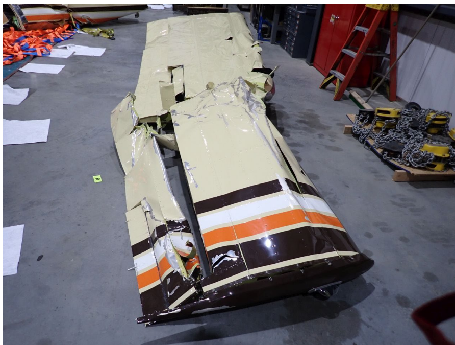
Figure 9 - Right wing (top) during post-recovery examination (NTSB photo)
