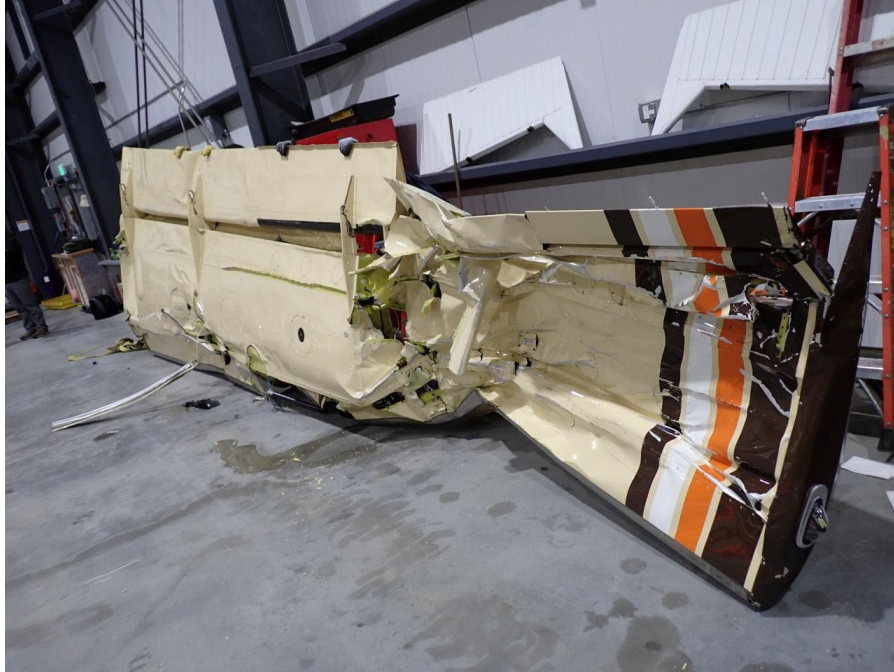
Figure 10 - Right wing (bottom) during post-recovery examination (Textron photo)
