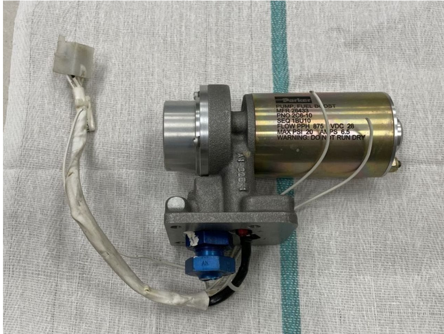
Figure 14 - Fuel boost pump (NTSB photo)
