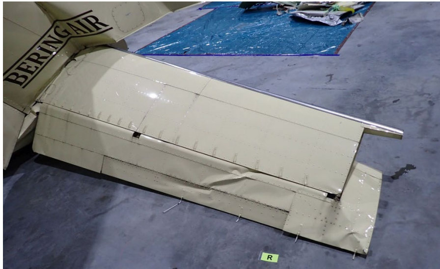
Figure 5 - Empennage during post-recovery examination (NTSB photo)
