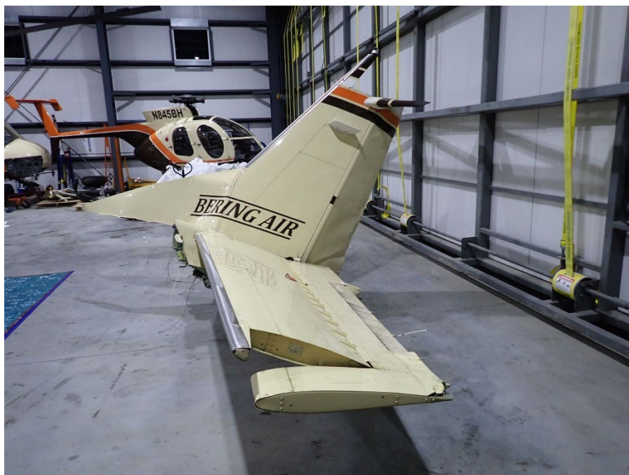
Figure 6 - Empennage during post-recovery examination (NTSB photo)
