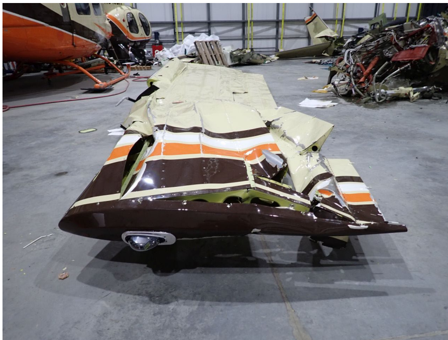
Figure 7 - Left wing (top) during post-recovery examination (NTSB photo)
