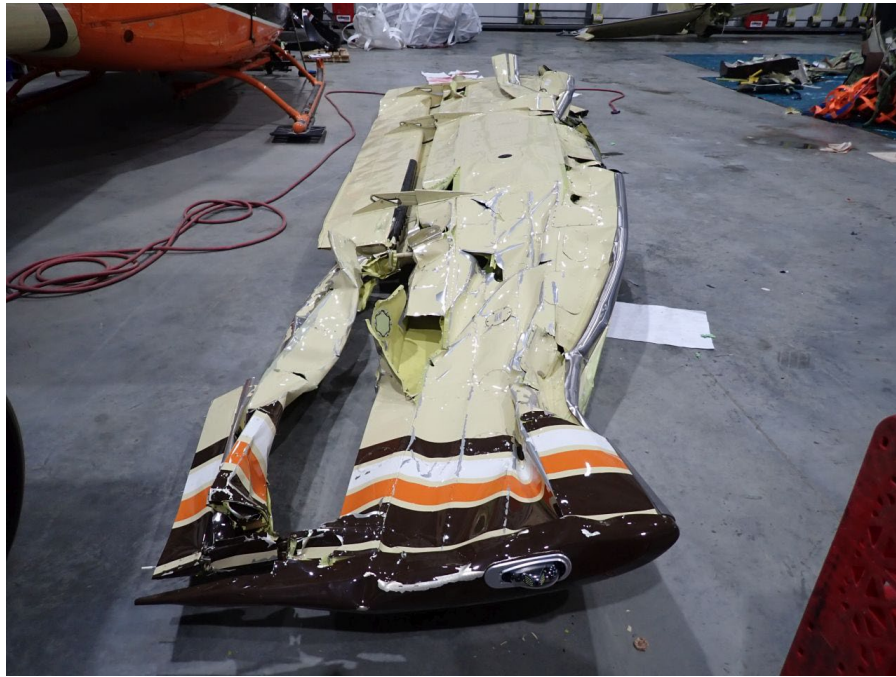
Figure 8 - Left wing (bottom) during post-recovery examination (NTSB photo)
