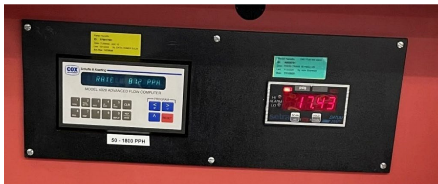
Figure 15 - Test bench readings at 872 pph test point (NTSB photo)
