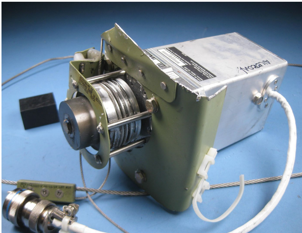
Figure 14. The airplane's aileron autopilot servo, the attached servo gearbox, and associated components.
