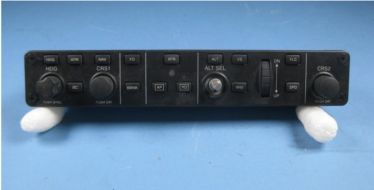
Figure 10. The front panel of the Autopilot Mode Control Unit, with the ALT SEL knob cover missing.
