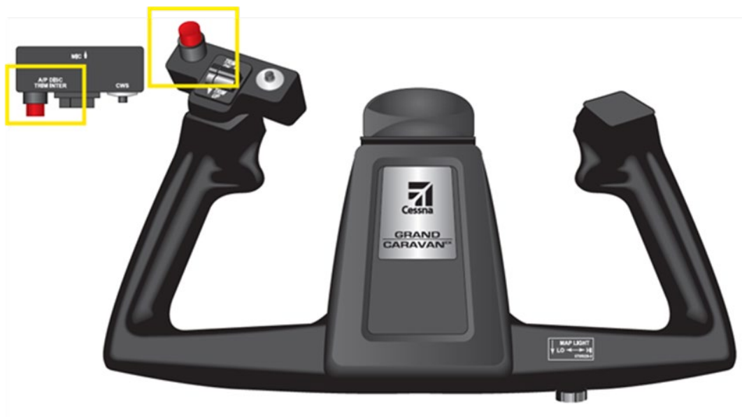
Figure 2. Airplane's control wheel with autopilot disconnect button highlighted in yellow box.(Figure courtesy of Textron)
