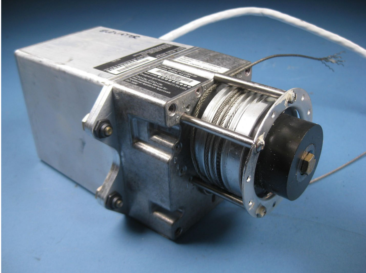
Figure 12. The airplane's autopilot elevator servo and attached servo gearbox.
