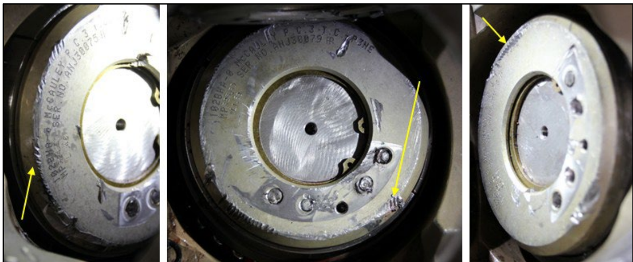
Figure 13. Blade Nos. 1 (Left), 2 (Center), and 3 (Right) Butt Damage
