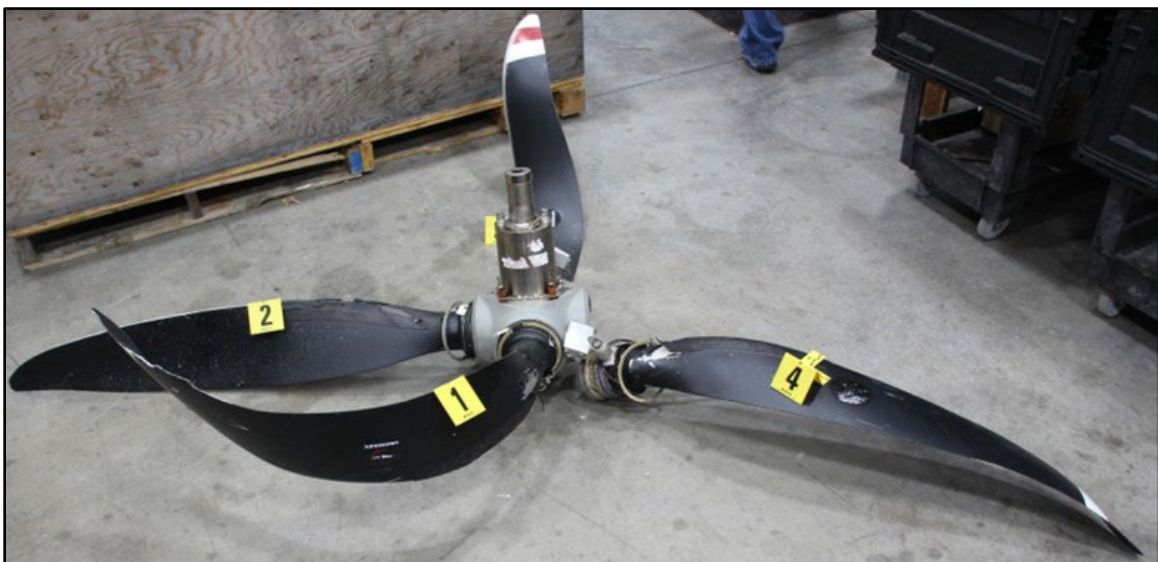
Figure 4. Propeller Removed - As Received
