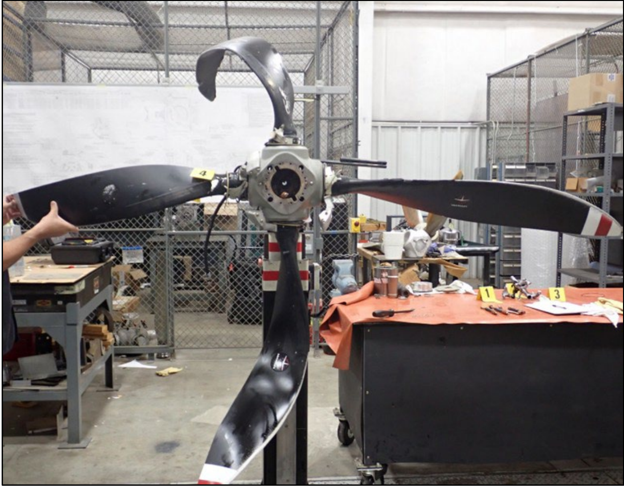
Figure 15. Propeller with Blades Aligned to Beta Rod Witness Marks
