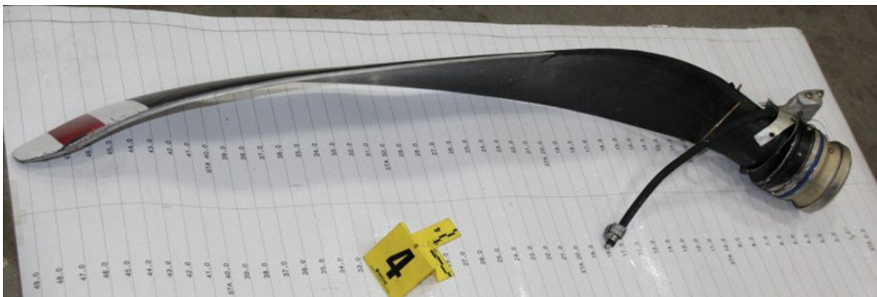
Figure 9. Separated No. 4 Blade
