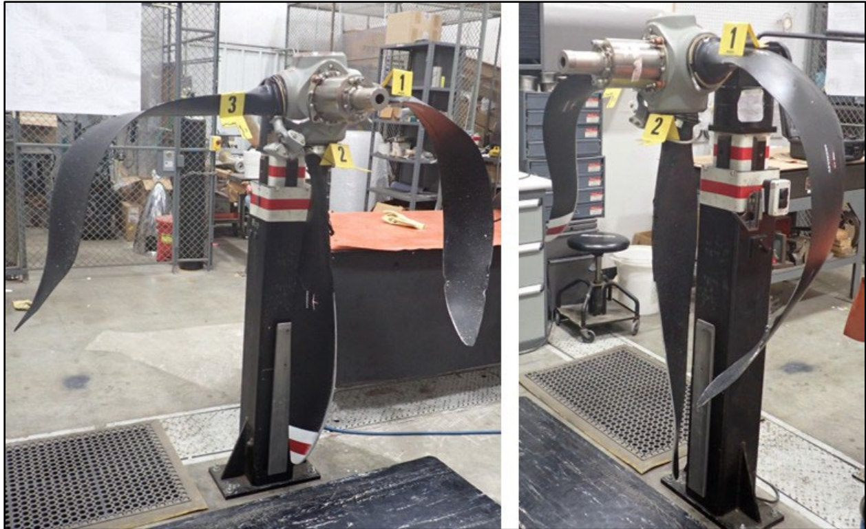
Figure 8. Propeller Mounted in a Test Stand
