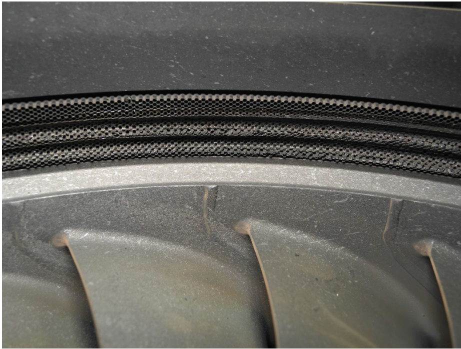
Photo 27 - PT Honeycomb Abradable Seal - Rotationally Scored
