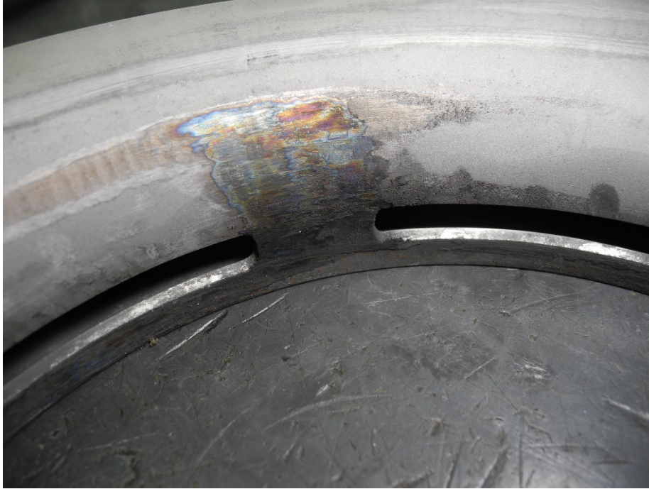
Photo 41 - Detail of Rotational Scoring on Impeller Shroud near Inducer
