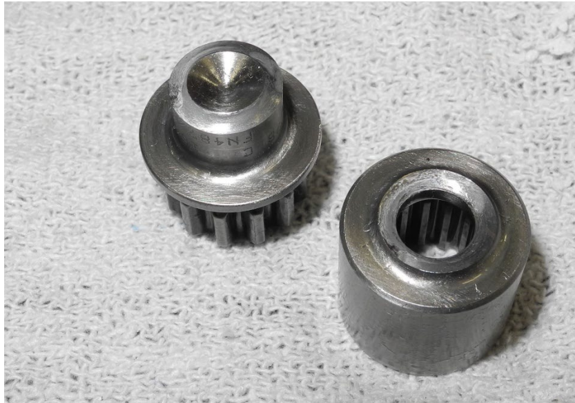
Photo 47 - Oil Pump Coupling Shaft - Sheared
