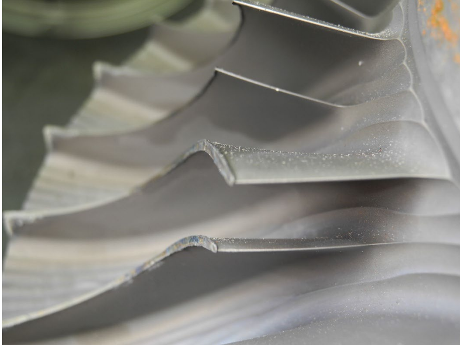
Photo 39 - Impeller Shroud Line - Rotational Scoring and Deformed, Rolled Material
