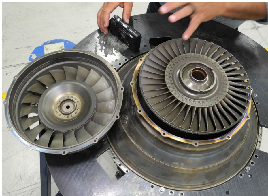
Photo 24 - PT Vane Ring and PT Wheel - Intact
