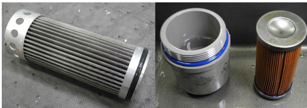
Photo 5 - Oil Filter (at Left) and Fuel Filter and Bowl (at Right)
