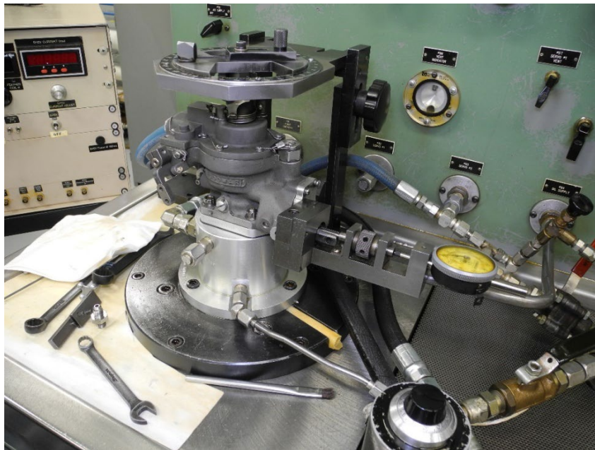
Photo 55 - CSU in Woodward Test Stand
