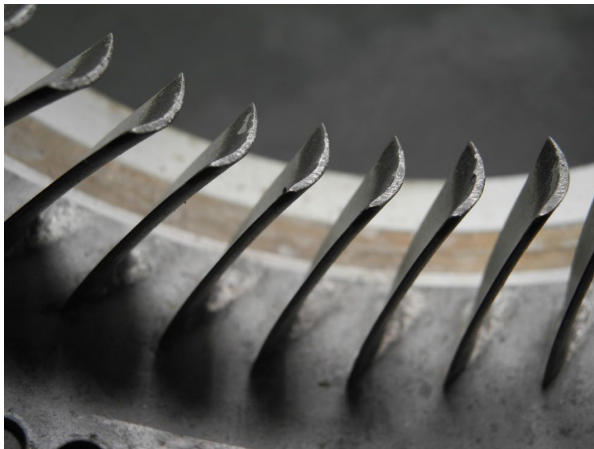
Photo 36 - 2 nd Stage Stator Vanes - Rubbing on Inner Tips
