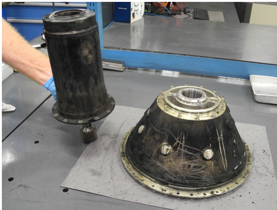
Photo 19 - PT Shaft Housing and RGB Aft Housing
