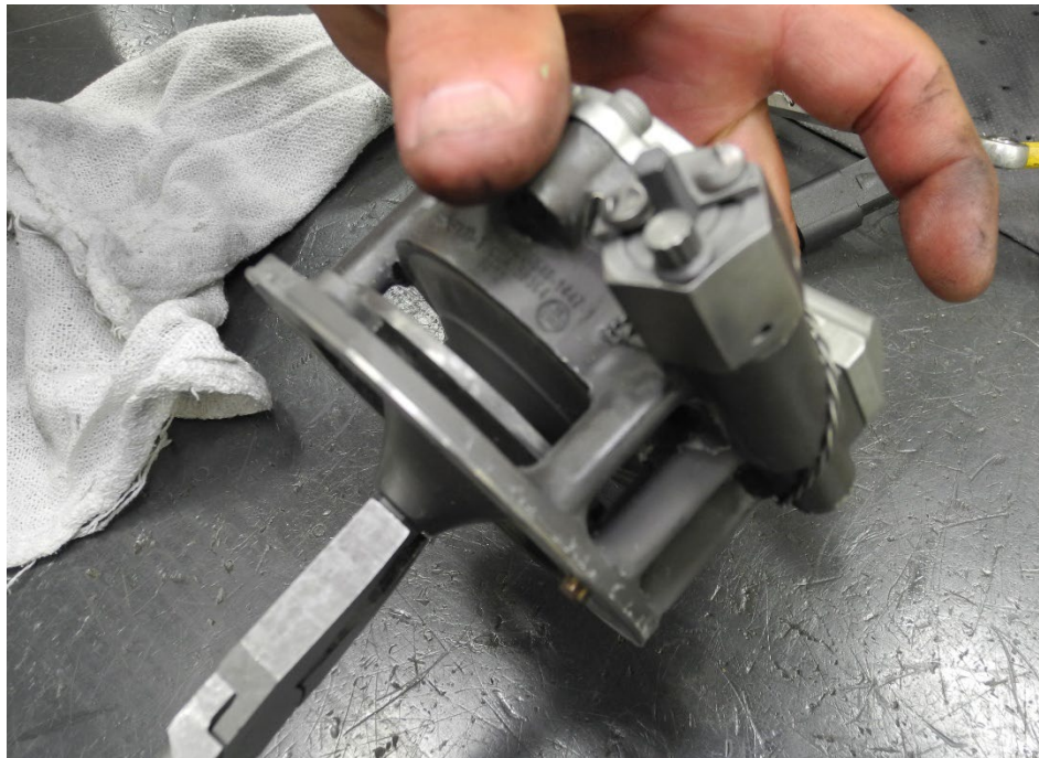
Photo 42 - Bleed Valve - Operational Confirmation
