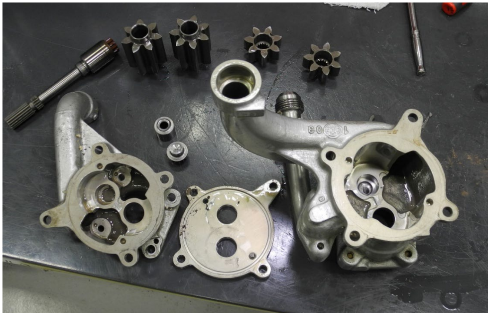
Photo 44 - External Oil Scavenge Pumps
