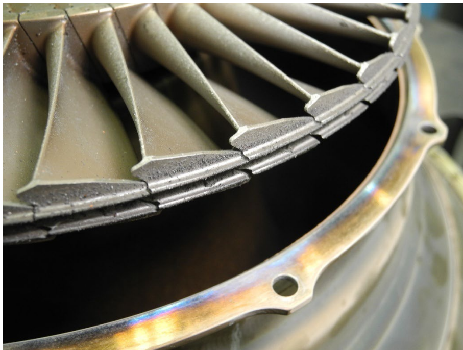
Photo 26 - Outer PT Blade Platforms - Rubbed
