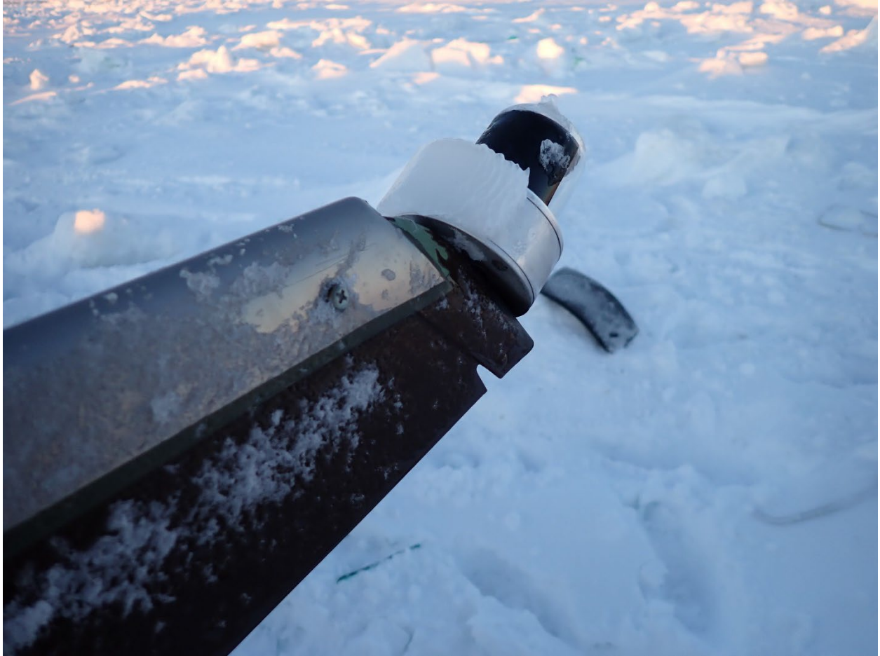
Figure 19. Accident wreckage tail section with icing noted on the airframe.
