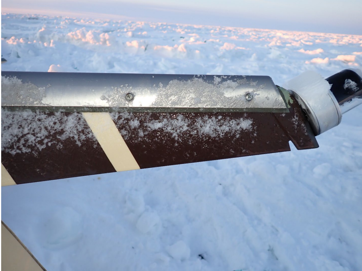
Figure 20. Accident wreckage tail section with icing noted on the airframe aft of the TKS porous membranes.
