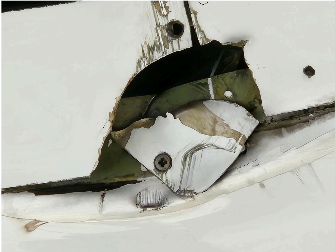
Photograph 2 - Damage to lower spar cap in the left wing(Courtesy of Operator)
