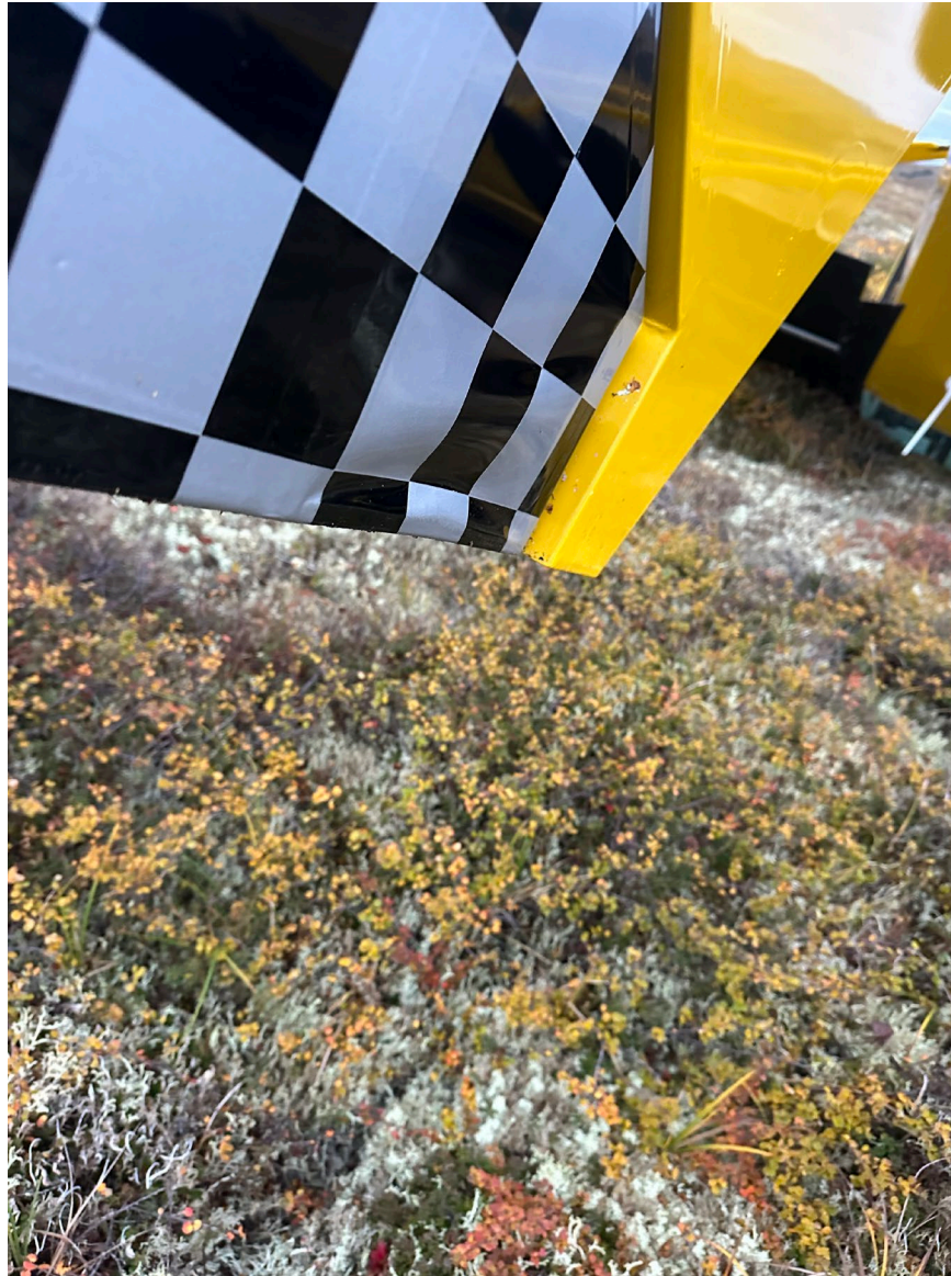
Photograph 2 - View of damage to the rudder. (Courtesy of the owner)
