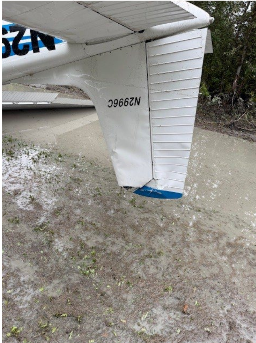
Photograph 4 - Damage to the vertical stabilizer and rudder (Courtesy of the pilot)
