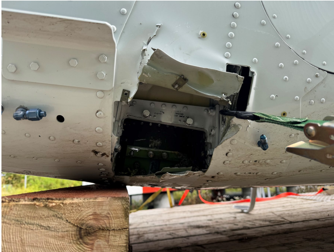
Photograph 3 - View of damage to the bottom of the fuselage (Courtesy of Federal Aviation Administration)
