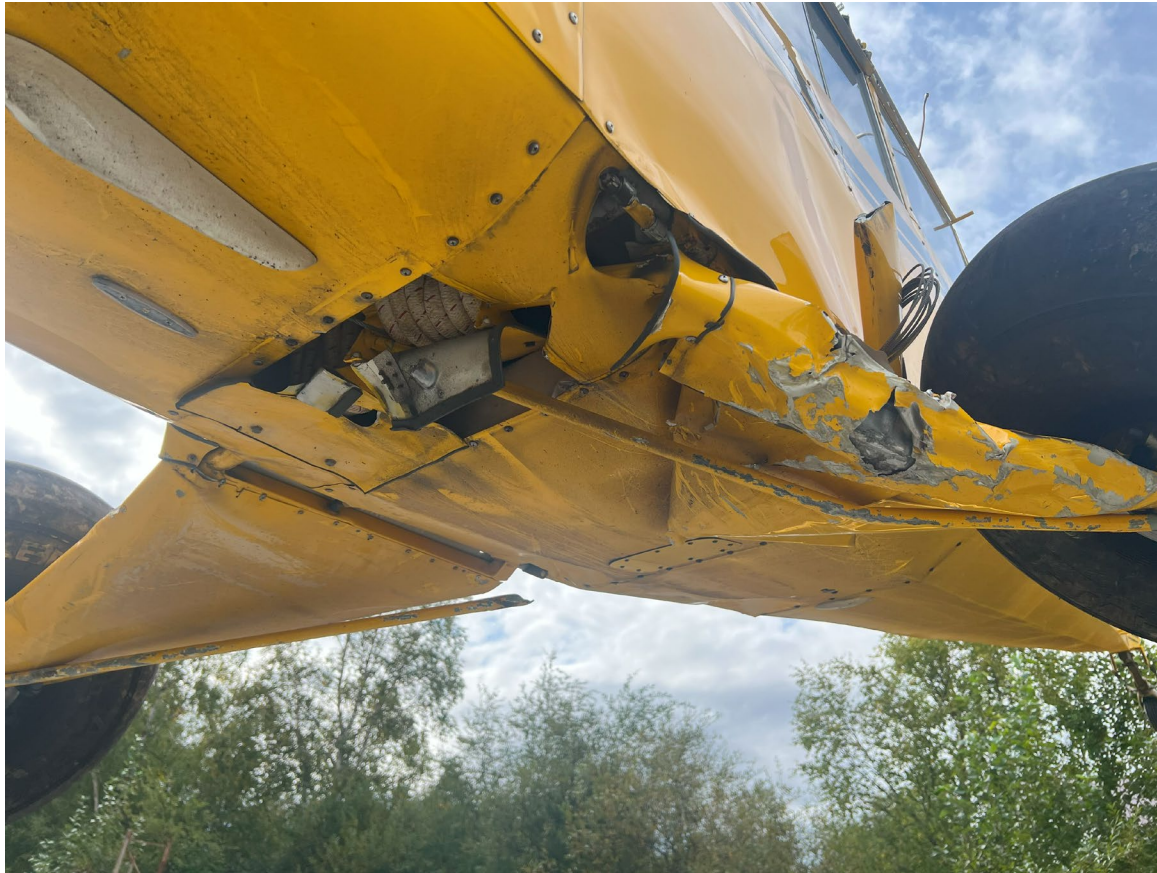
Photograph 2 - View of landing gear. Bungees still attached, fractures from overload from hard landing.
