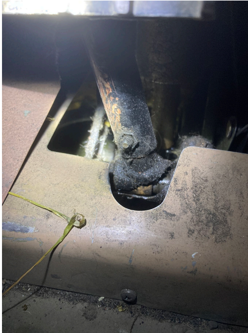
Photograph 3 - View of the failure of the left rudder assembly (Courtesy of FAA)
