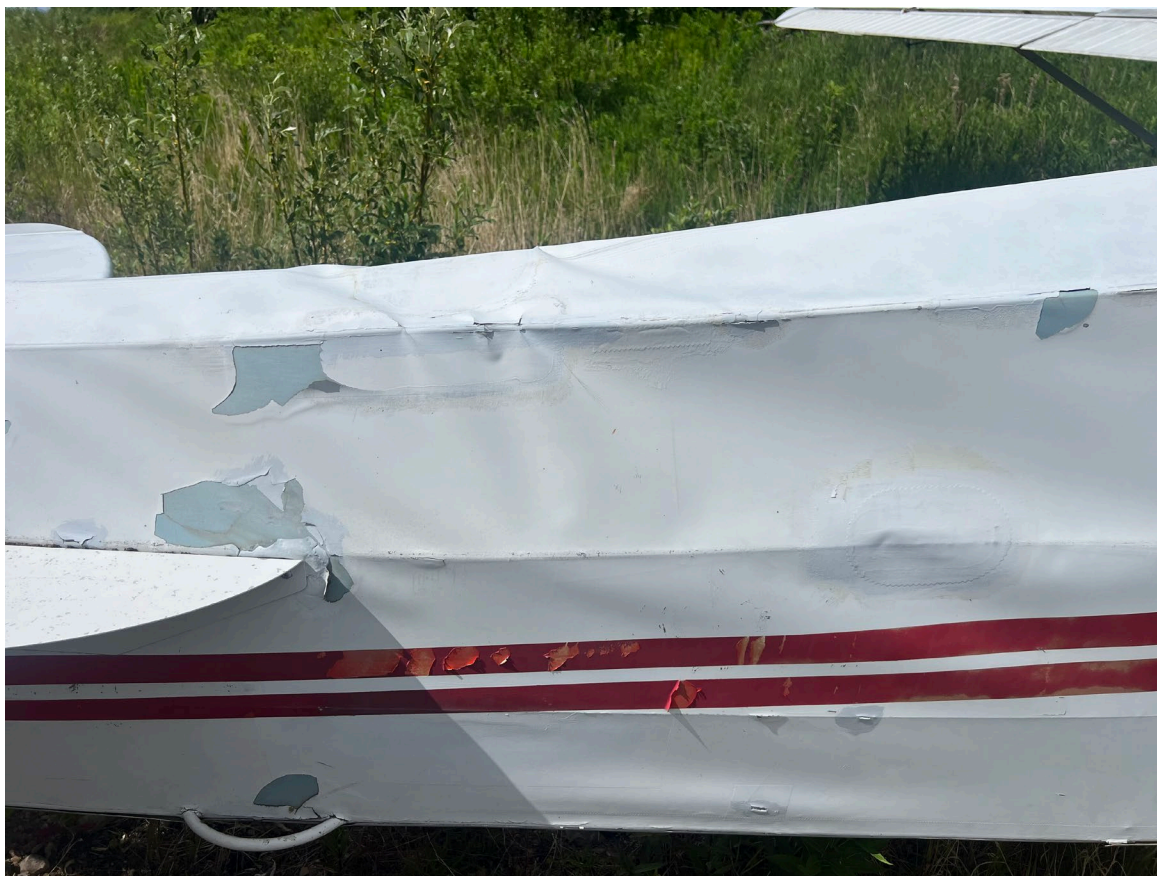
Photograph 3 - Image of damage to tail section (Courtesy of Owner)
