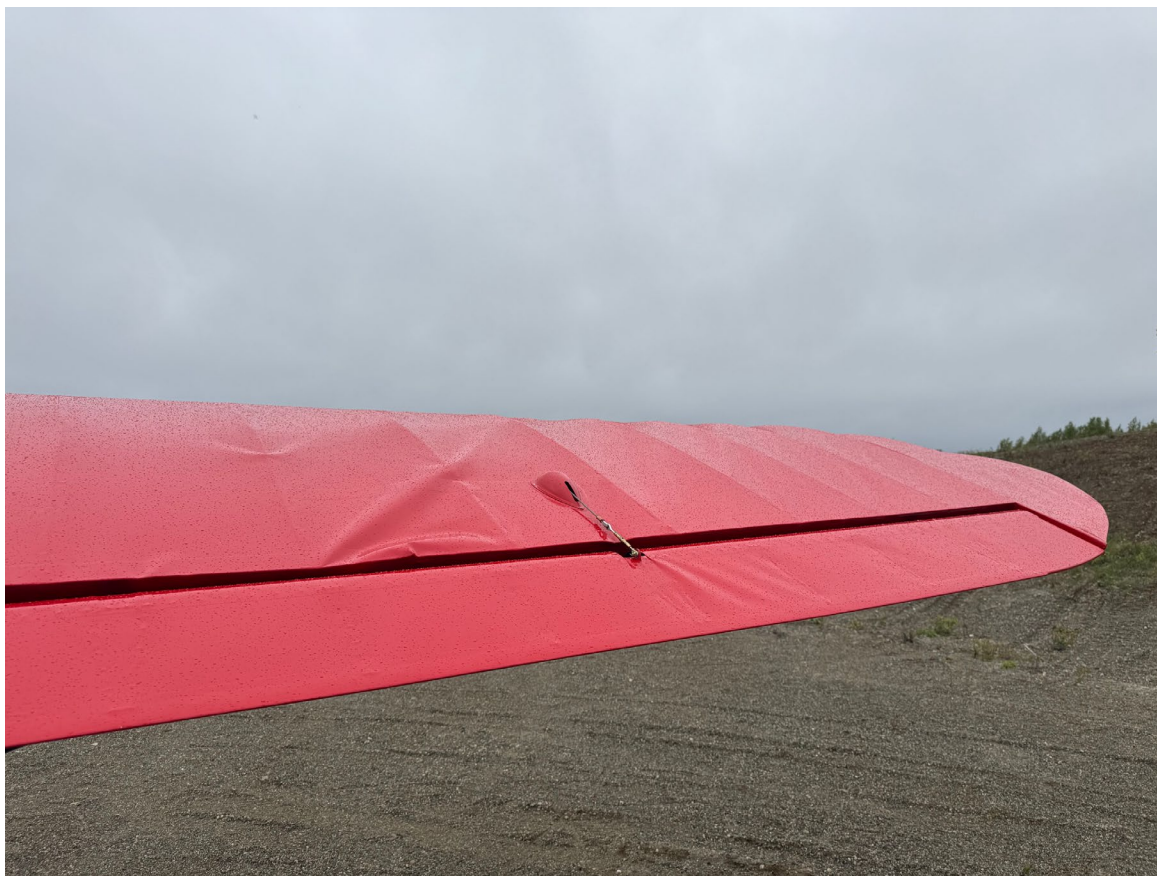
Photograph 2 - View of damage to the top of the right wing. (Courtesy of pilot)
