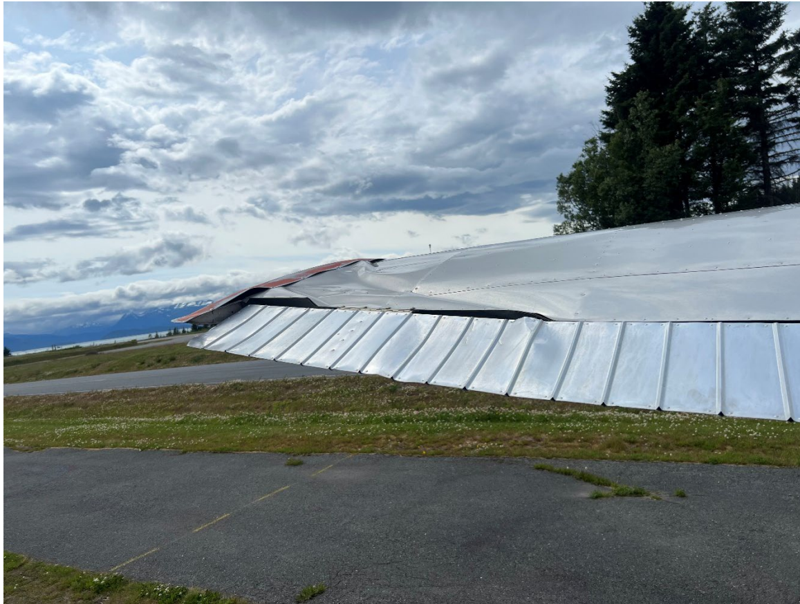
Photograph 1 - Image of damage to left wing (Courtesy of Owner)
