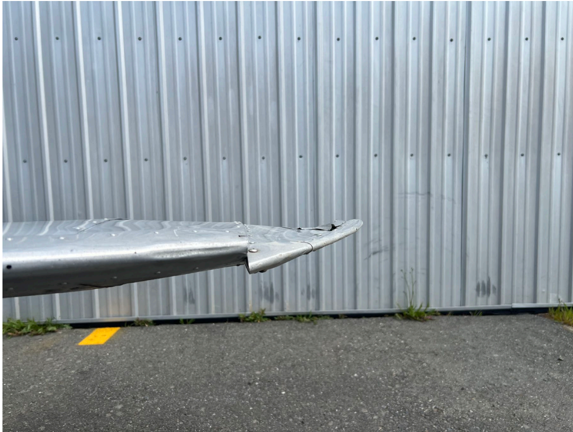
Photograph 2 - Image of damage to right wing tip (Courtesy of Owner)
