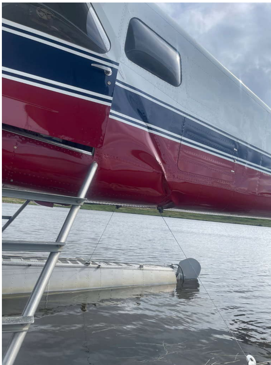
Photograph 2 - Image of damage to airplane fuselage (Courtesy of Owner)
