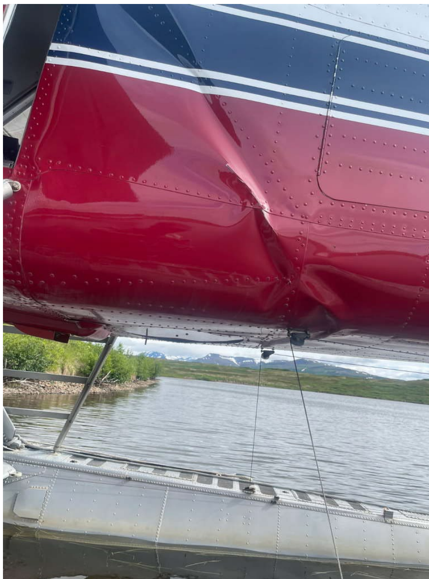
Photograph 1 - Image of damage to fuselage (Courtesy of Owner)
