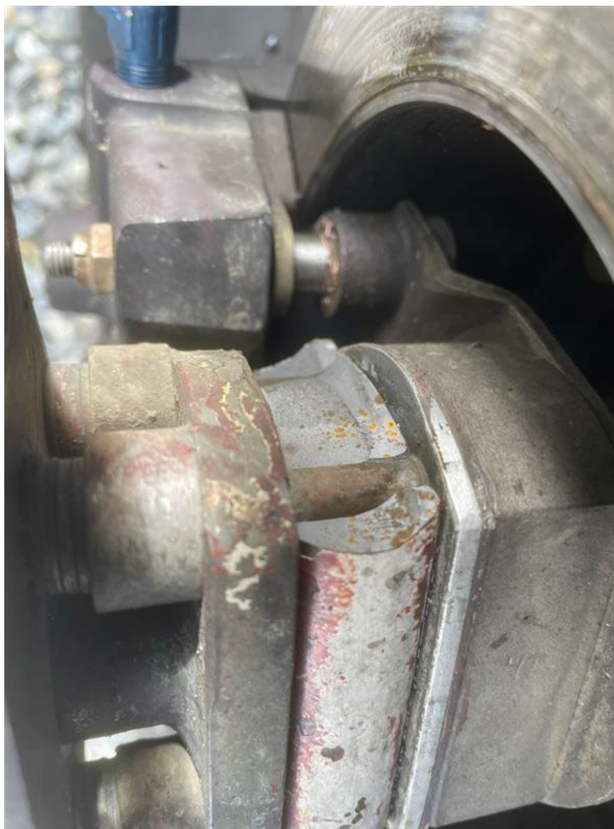
Photograph 3 - Fractured main landing gear spring attached to wheel axle (Courtesy of Owner)
