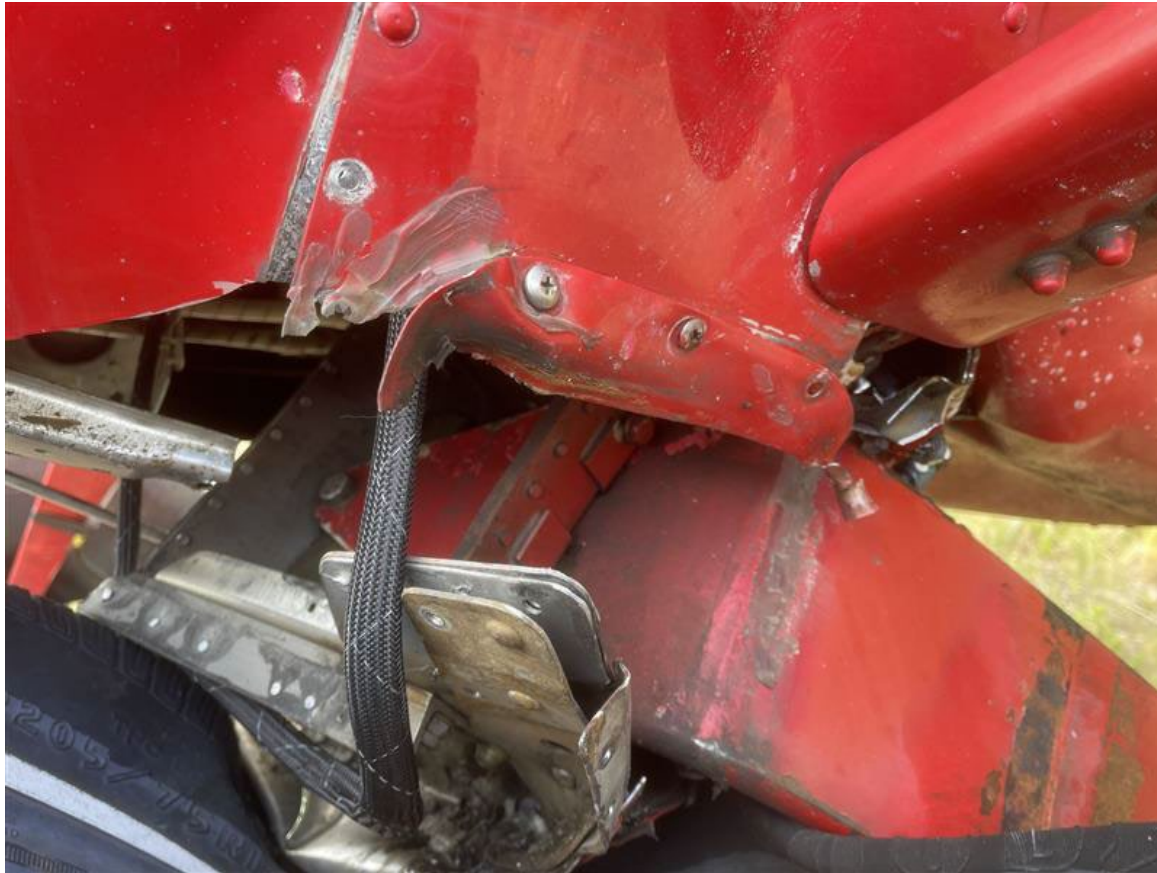
Photograph 2 - Main landing gear spring to fuselage attach point (Courtesy of Owner)
