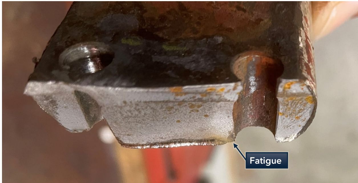
Figure 1. Fatigue crack at the inboard corner of the forward hole (Photo by owner).
