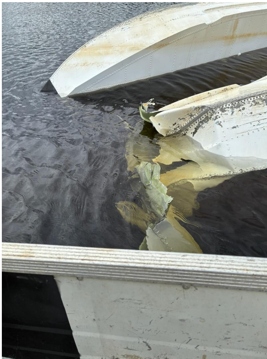
Photograph 2 - View of damage to the floats (Courtesy of FAA)
