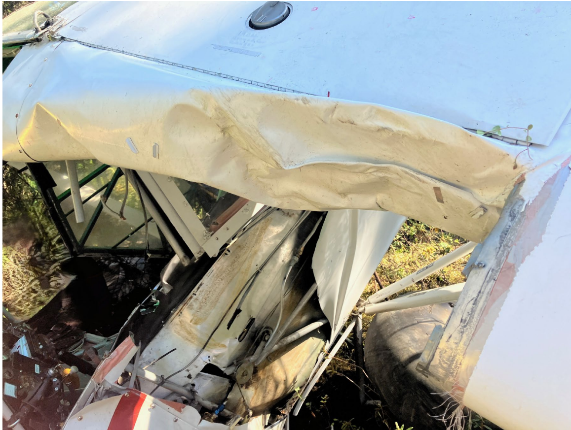
Photograph 2 - Image of damage to left wing and fuselage (Courtesy of Alaska State Troopers)
