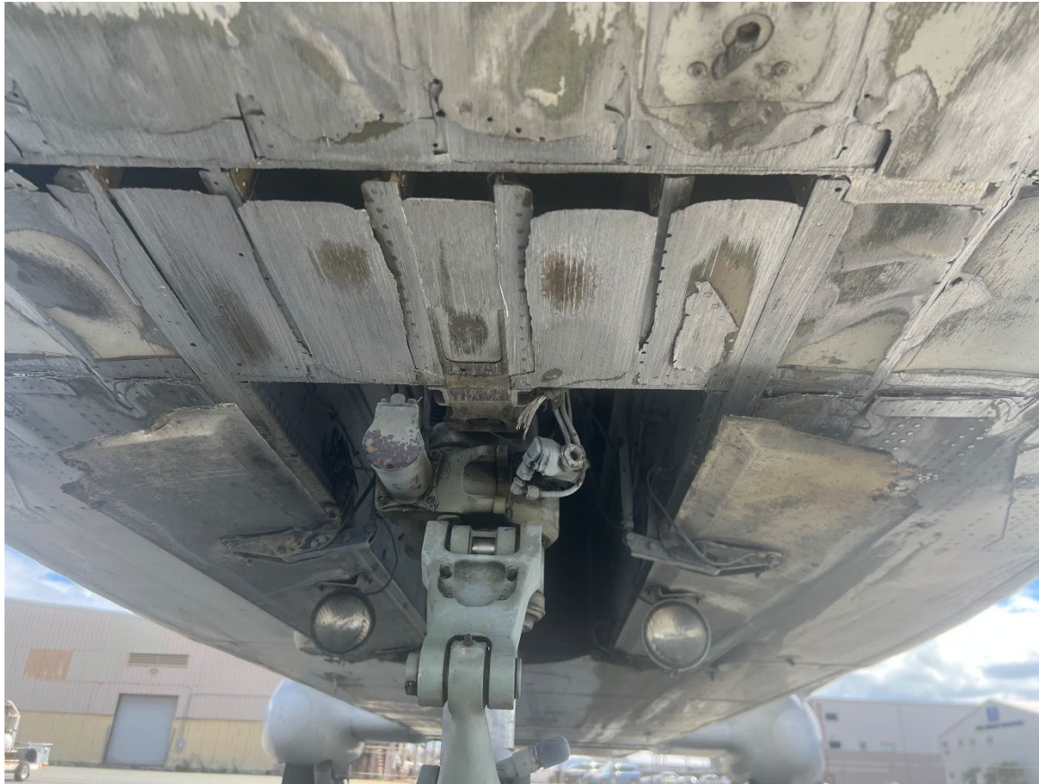
Photograph 2 - Image of damage to belly of airplane (Courtesy of operator)
