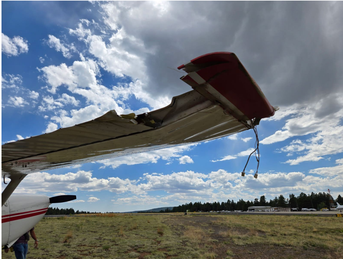
Photograph 1 - Image of damage to right wing (Courtesy of Airport Manager)
