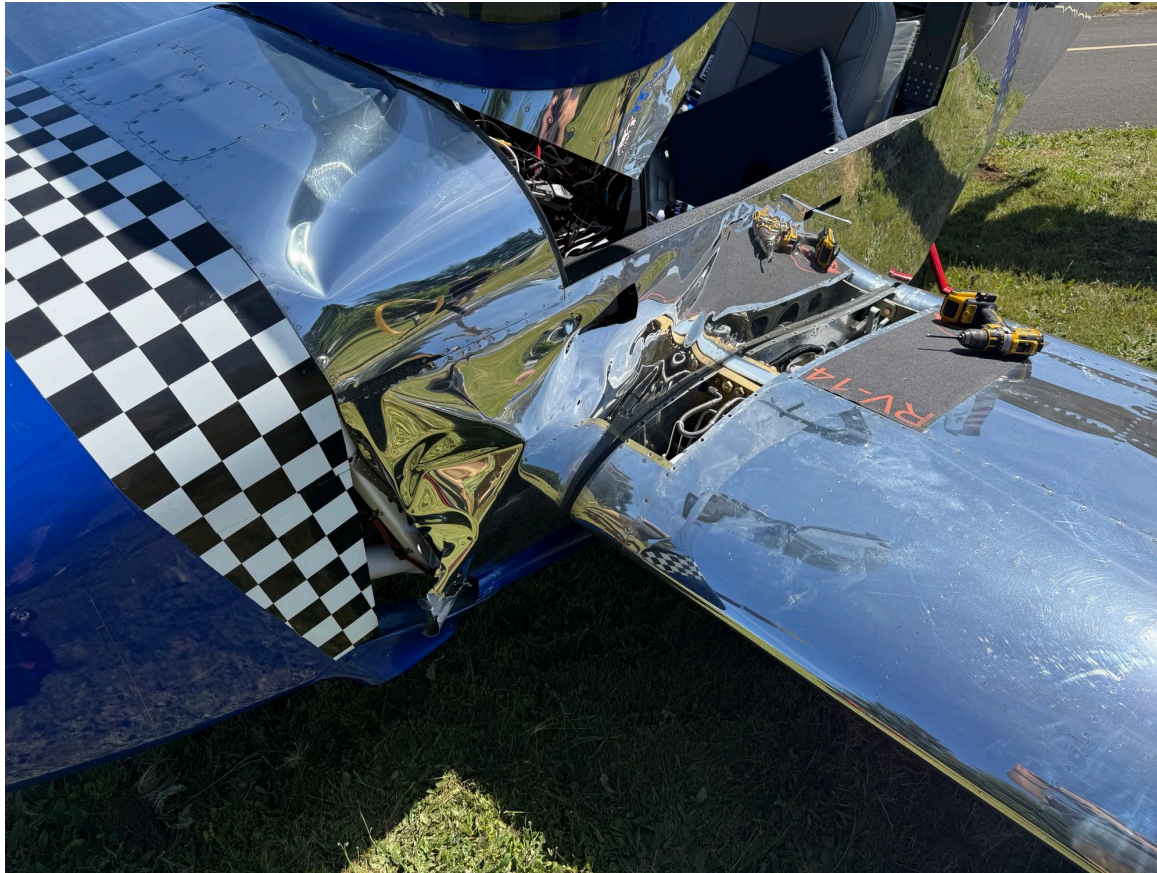
Photograph 2 - Image of left wing attachment point (Courtesy of owner)
