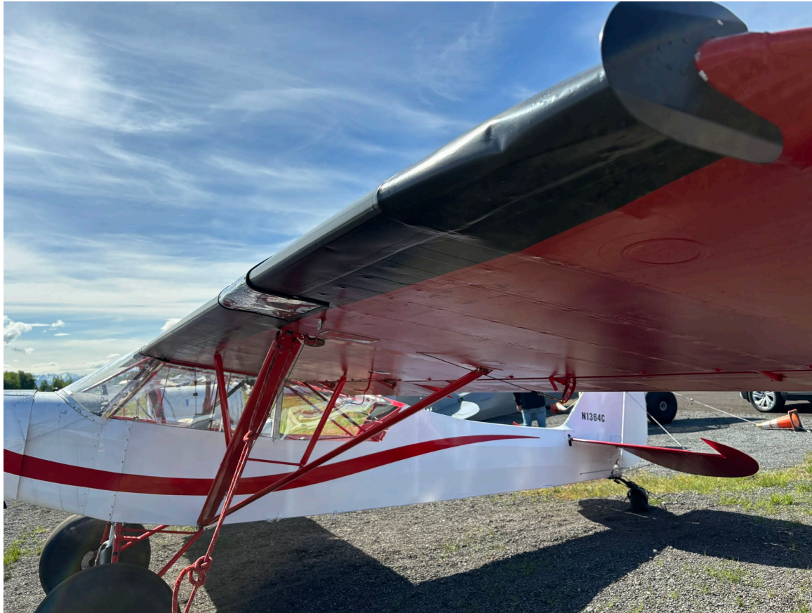
Photograph 2 - View of damage to left leading edge. (Courtesy of FAA)
