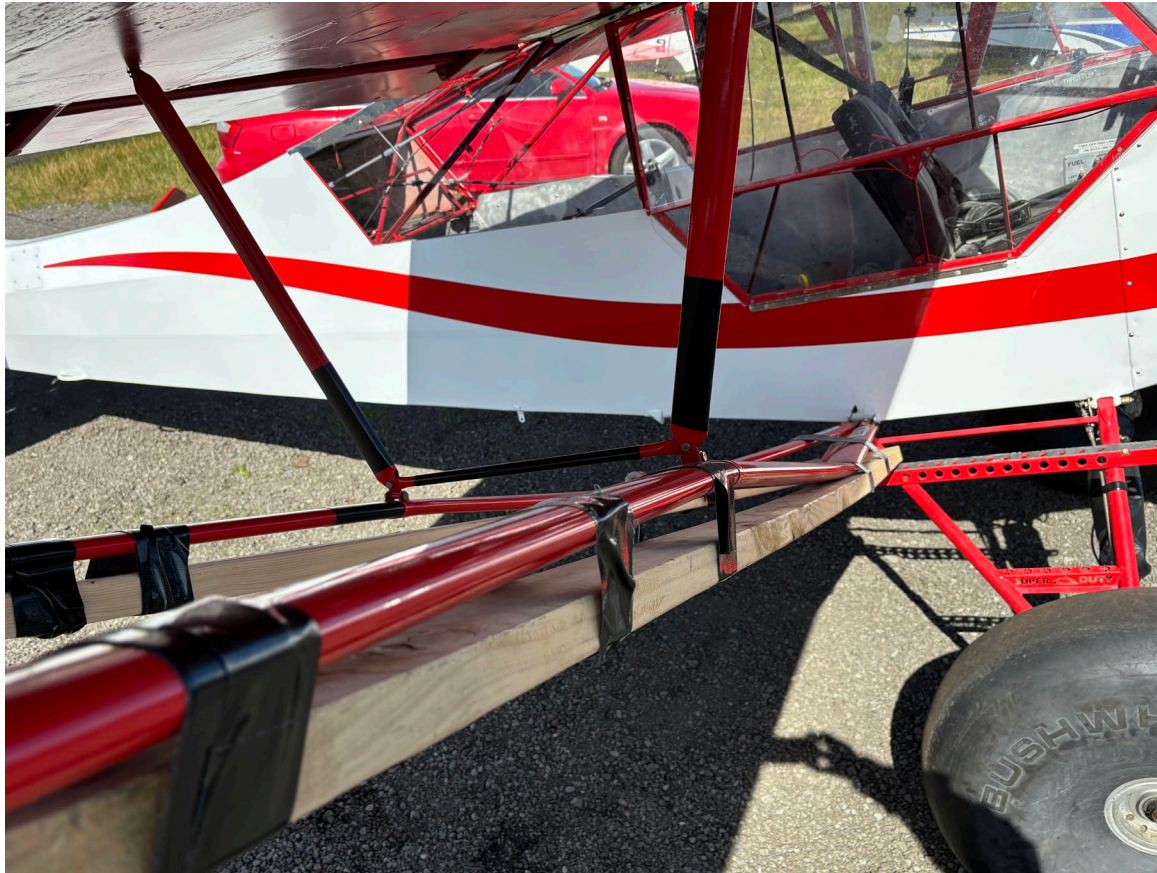
Photograph 1 - View of damage to right strut. (Courtesy of FAA)
