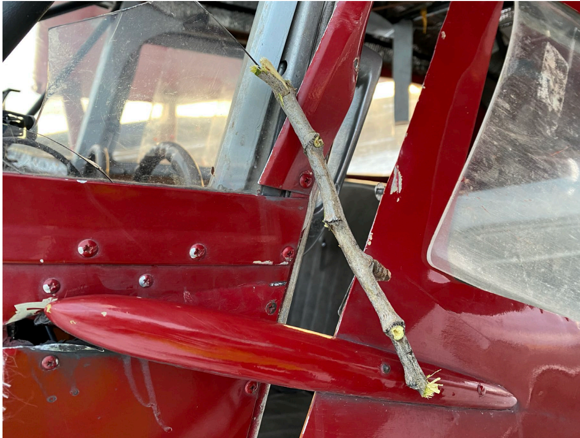
Photograph 3 - View of a stick lodged in the airframe around the windscreen (Courtesy of airfield manager)
