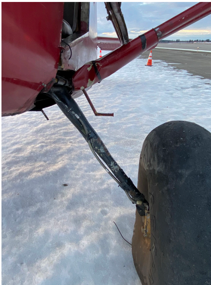
Photograph 4 - View of damage to left strut. (Courtesy of airfield manager)
