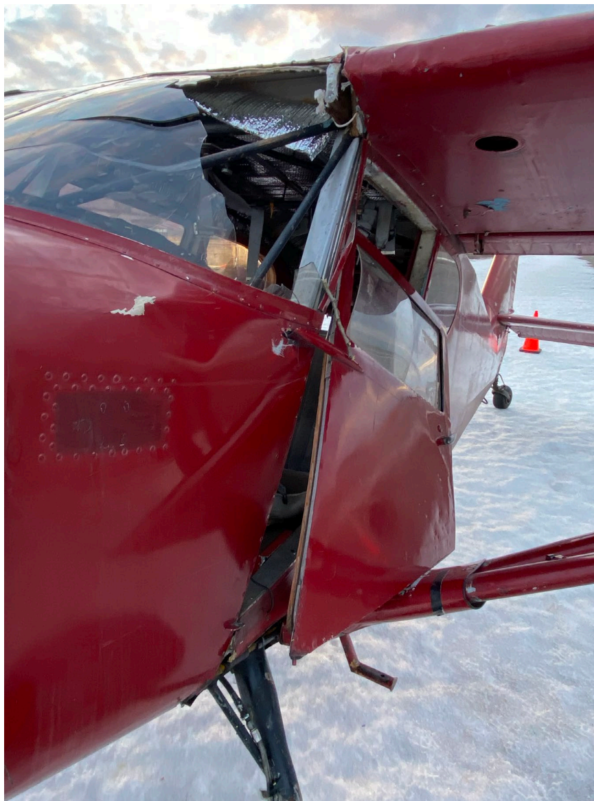
Photograph 2 - Damage to windscreen and left side of fuselage (Courtesy of airfield manager)
