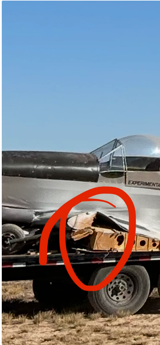
Photograph 2 - Damage to the left side of the accident airplane (Courtesy of the owner)
