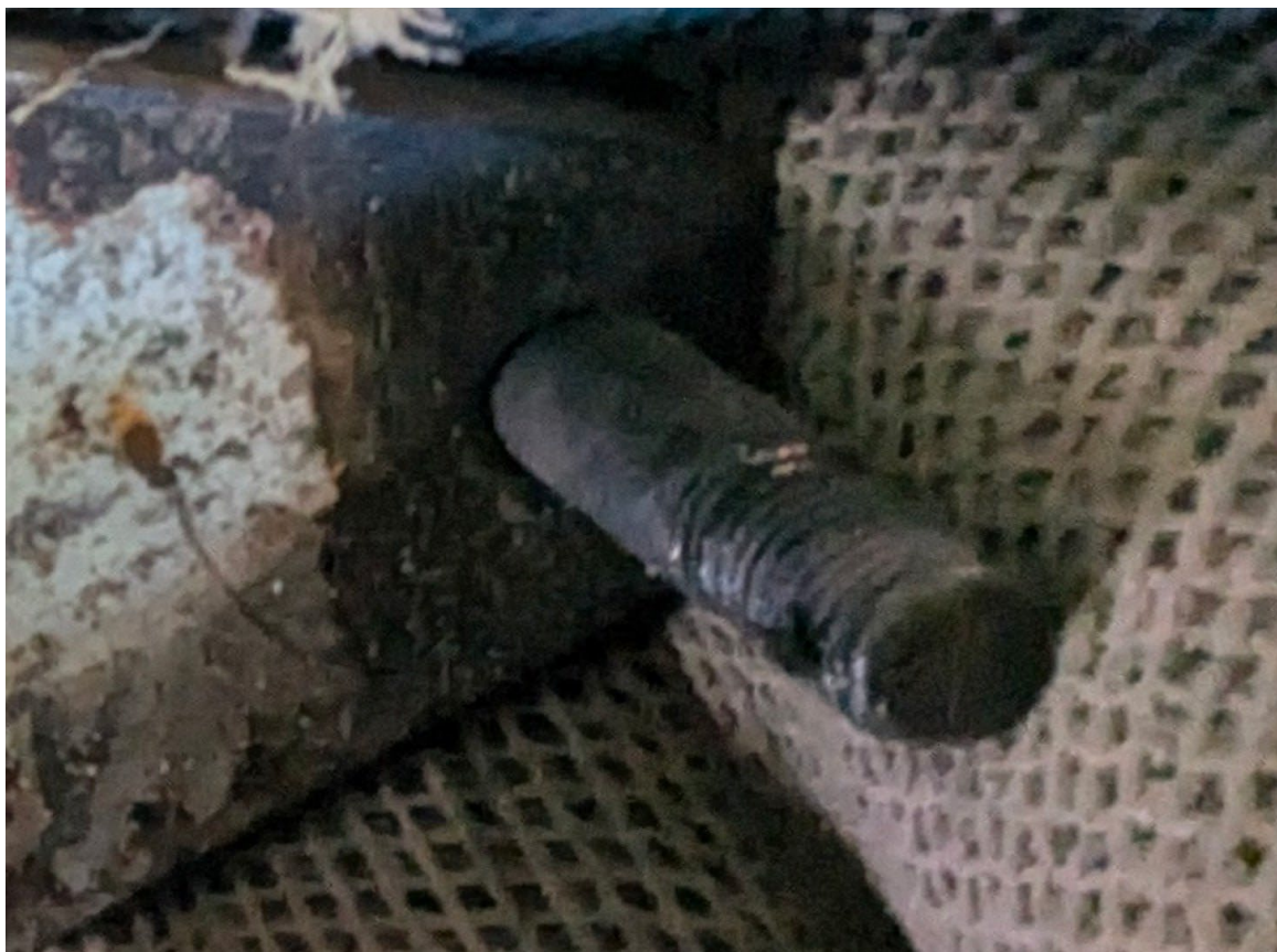
Photograph 3 - Bolt as found after accident in landing gear (Courtesy of Owner)
