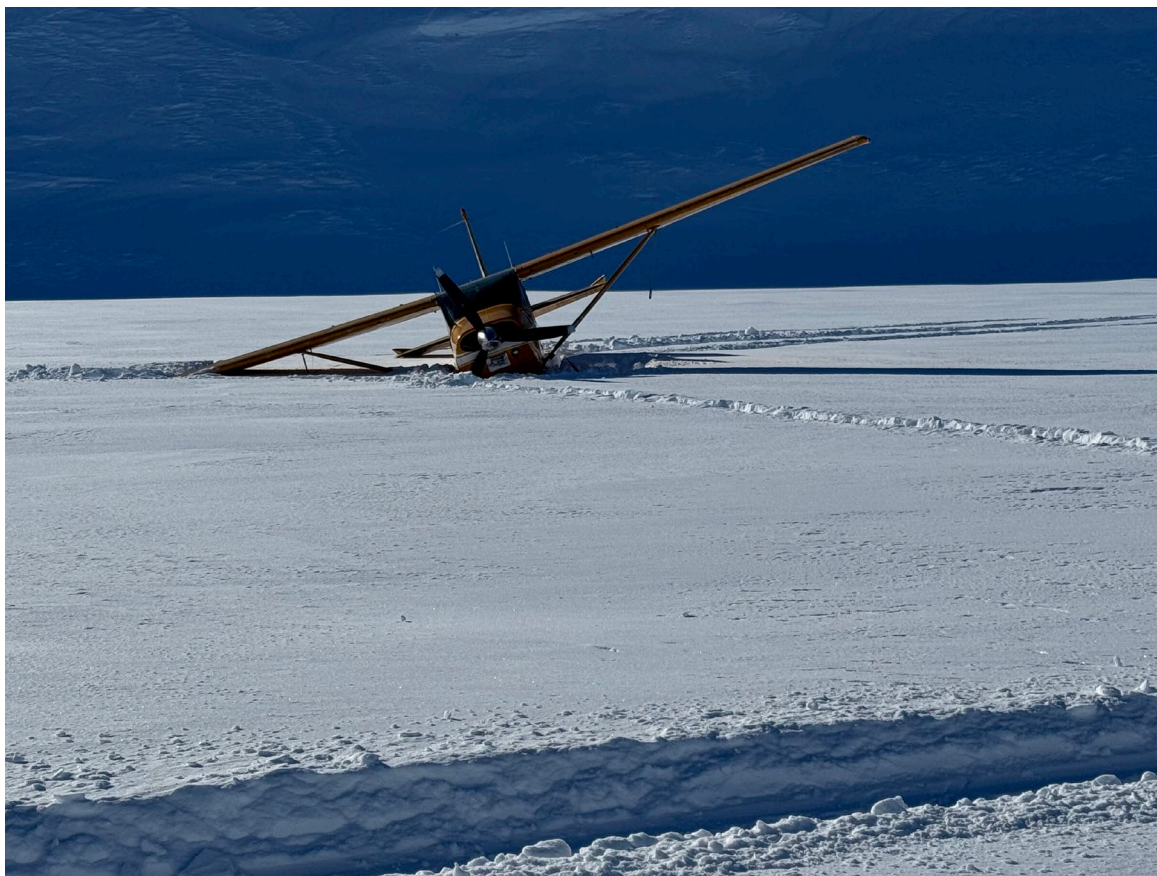
Photograph 1 - Airplane with collapsed gear leg (Courtesy of Owner)
