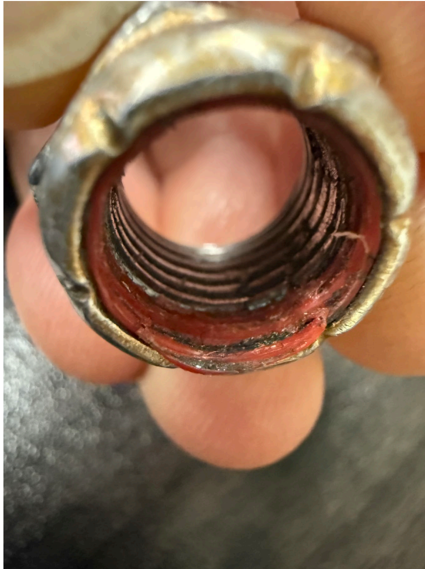
Photograph 4 - Fiber locking nut from landing gear assembly (Courtesy of NTSB)
