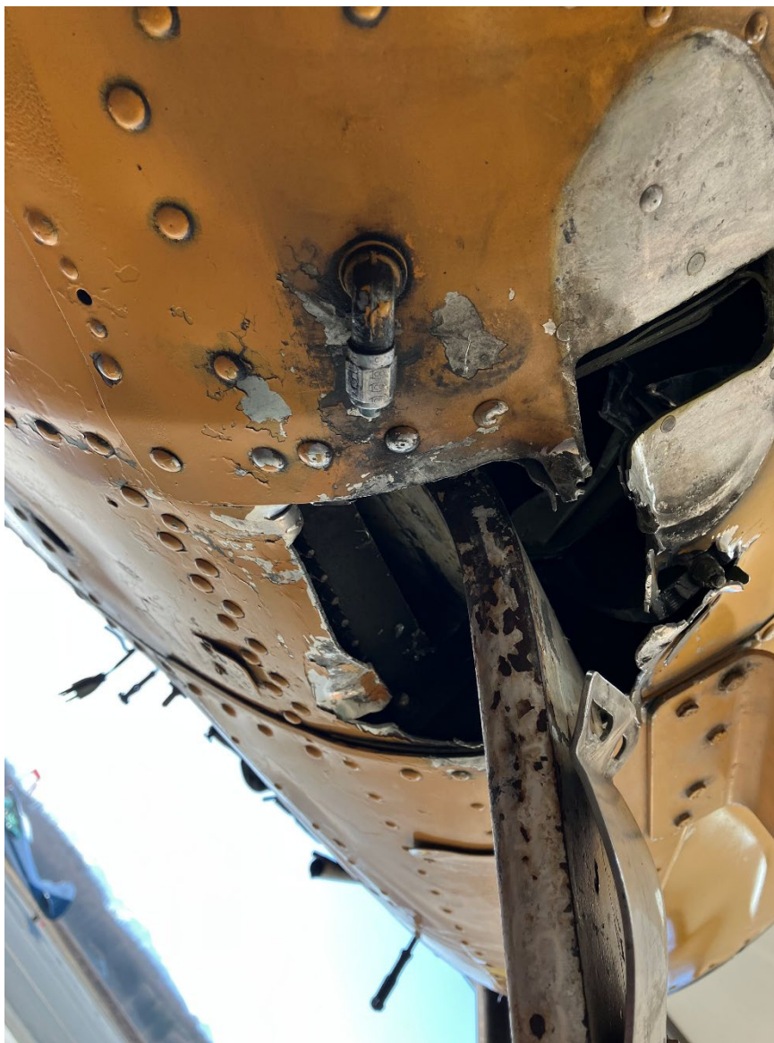
Photograph 2 - Damage to landing gear box assembly (Courtesy of owner)
