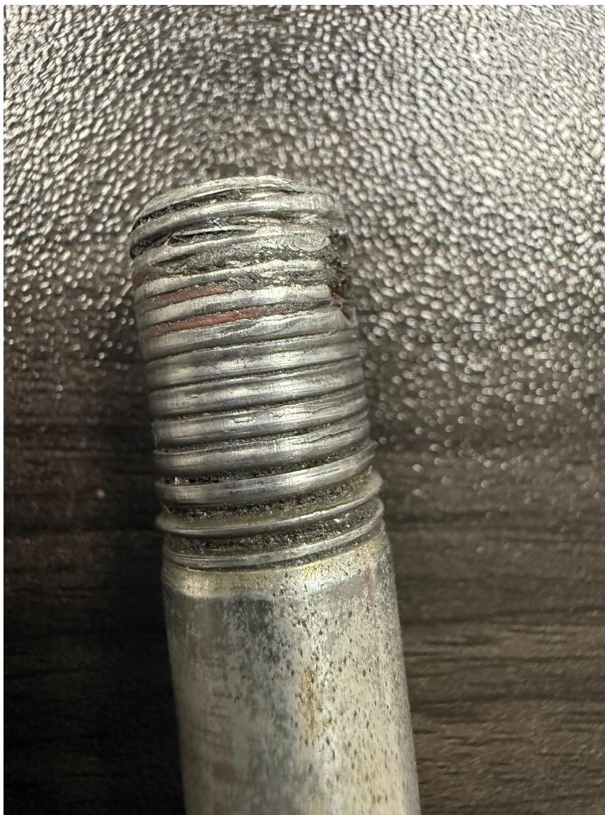
Photograph 5 - Bolt from landing gear assembly (Courtesy of NTSB)
