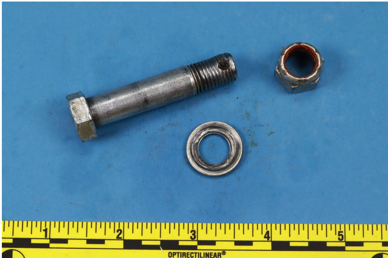
Figure 1. Main landing gear bolt, nut and washer as received.
