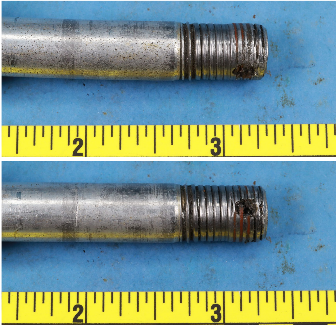
Figure 3. Two views of the worn threads on the bolt. The threads on the end contain remnants of the nylon locking insert from the nut.
