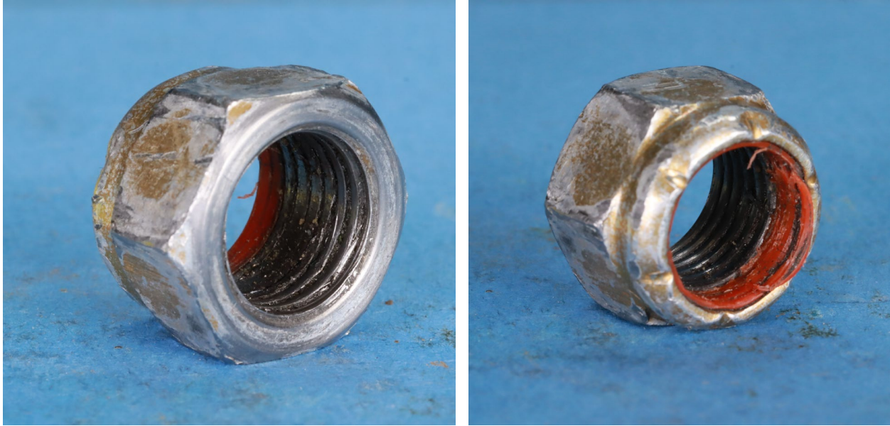
Figure 4. Locking nut exhibiting worn internal threads and a damaged nylon insert.
