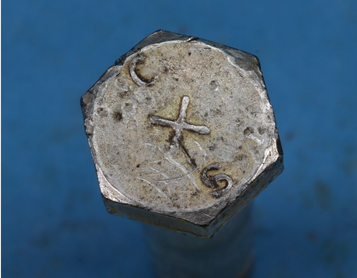
Figure 2. Markings on the bolt head.
