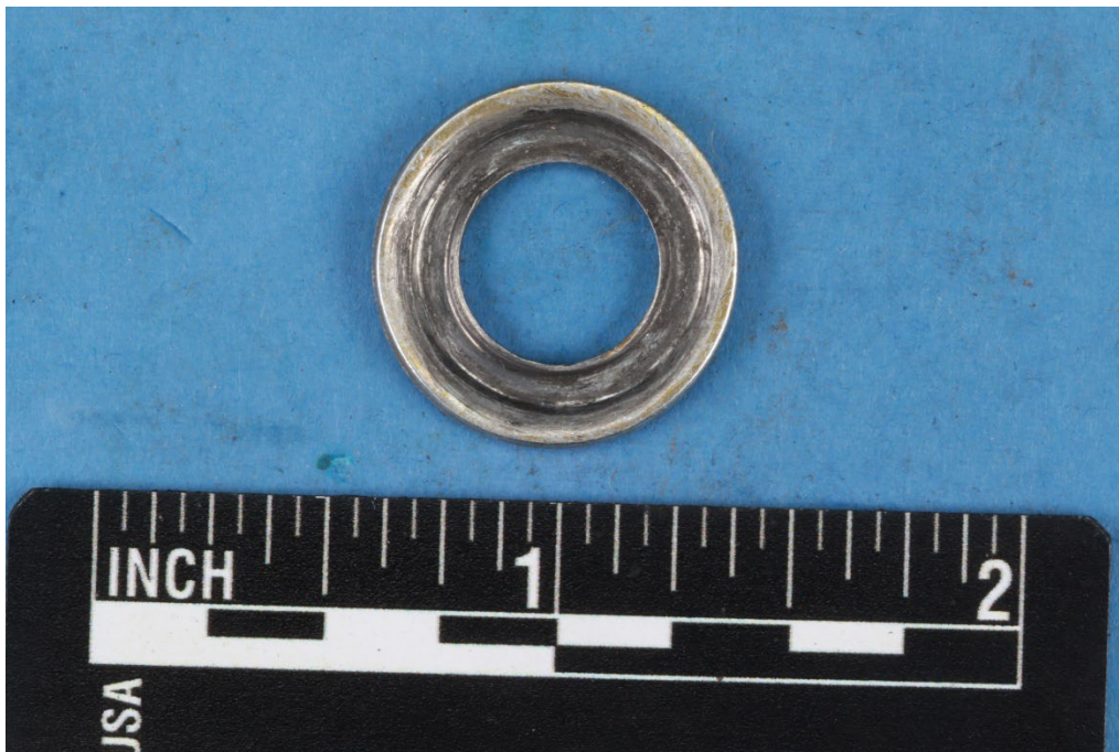
Figure 5. Flat washer with wear groove.
