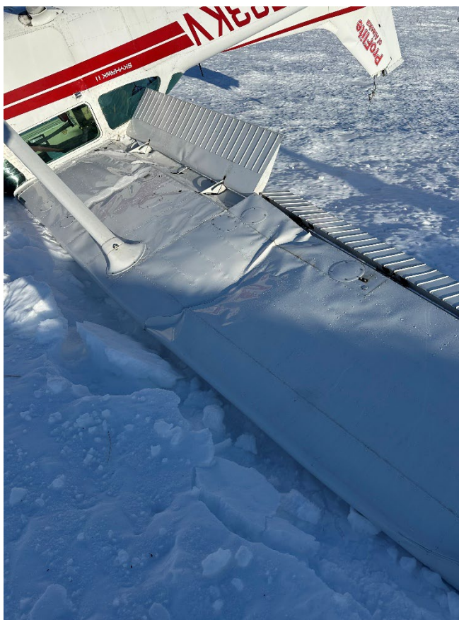
Photograph 2 - Damage to right wing (Courtesy of Owner)
