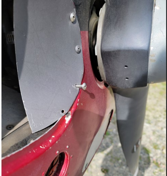
Figure 4 Screw backing out of nose bowl of accident airplane.
