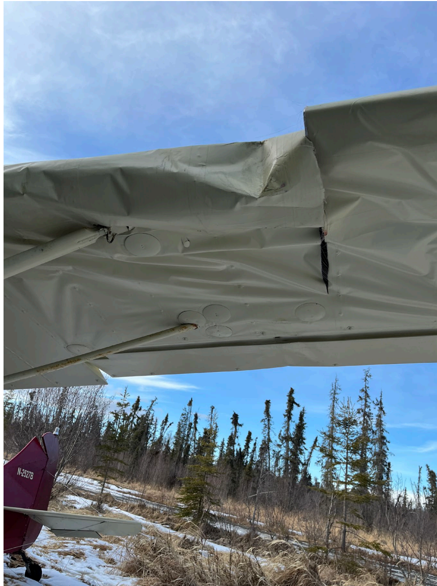
Photograph 2 - Damage to left wing (Courtesy of FAA)
