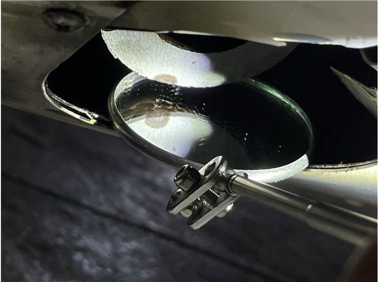
Figure 9 View of the fracture surface of landing gear that is still attached to the airplane.
