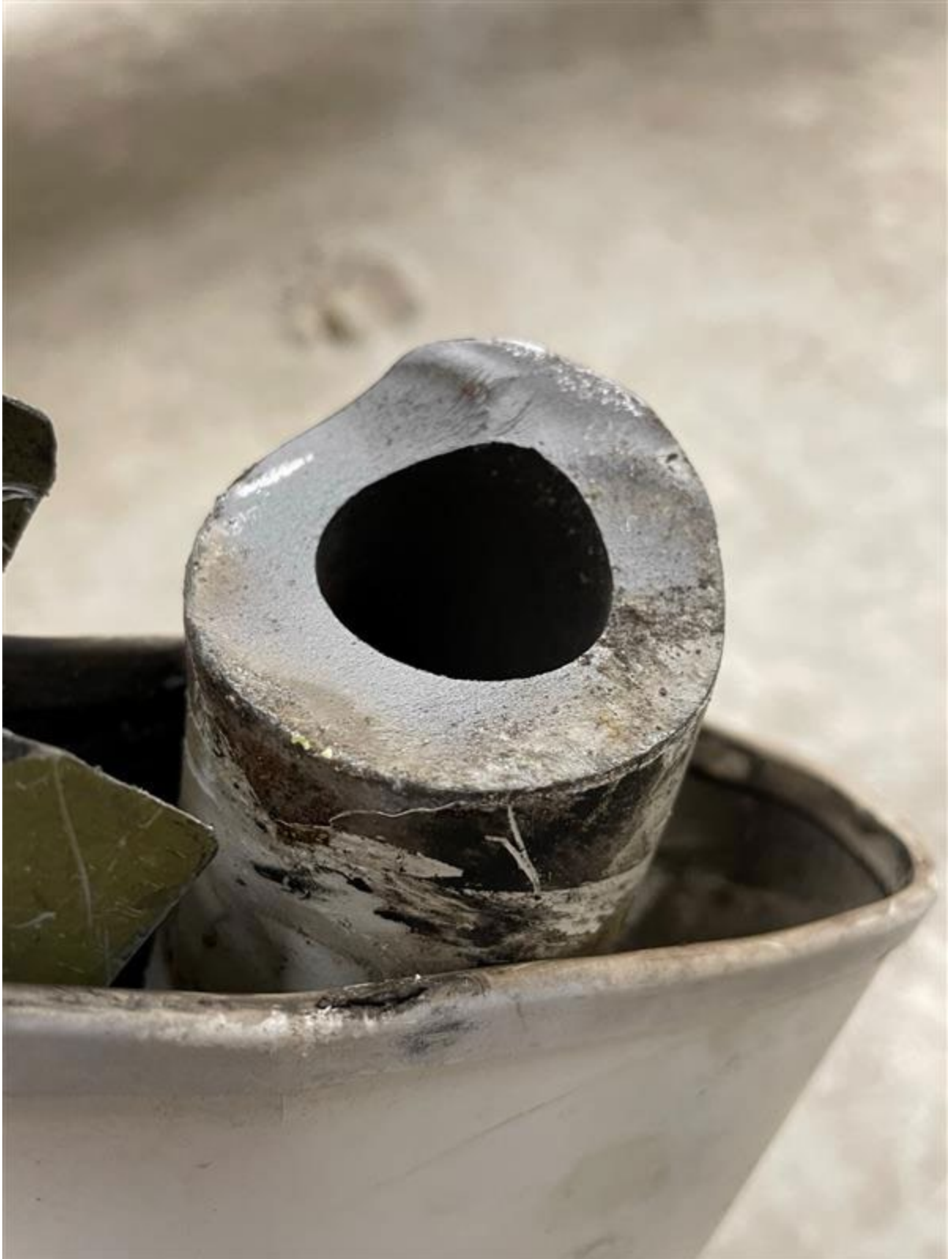
Figure 6 Fracture surface of the right landing gear.
