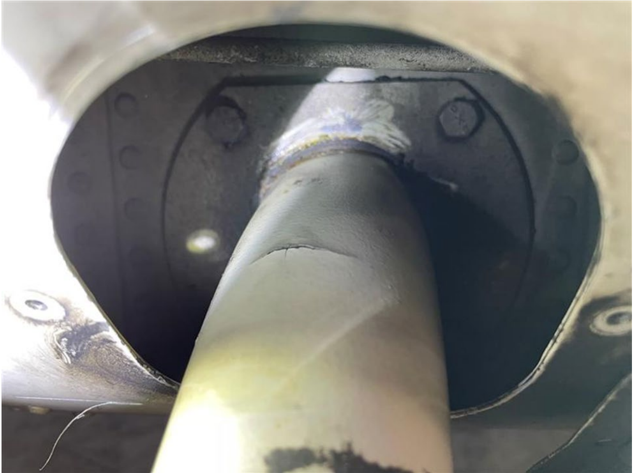
Figure 11 View of the left landing gear near the fuselage attachment point. Corrosion is visible in the same location as the fracture on the right-side landing gear.
