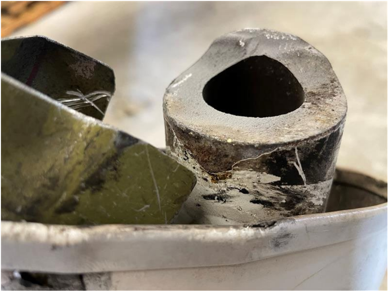
Figure 8 Fracture surface of the right landing gear.
