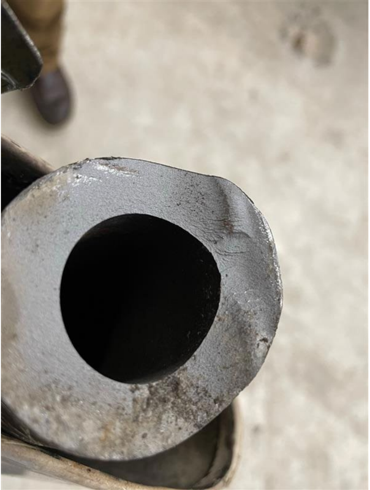
Figure 7 Fracture surface of the right landing gear.
