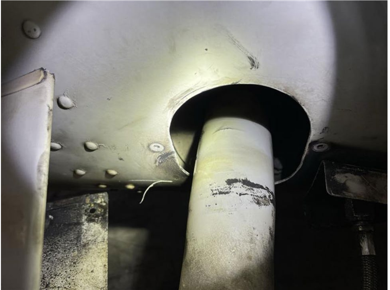
Figure 12 View of the left landing gear near the fuselage attachment point. Corrosion is visible in the same location as the fracture on the right-side landing gear.
