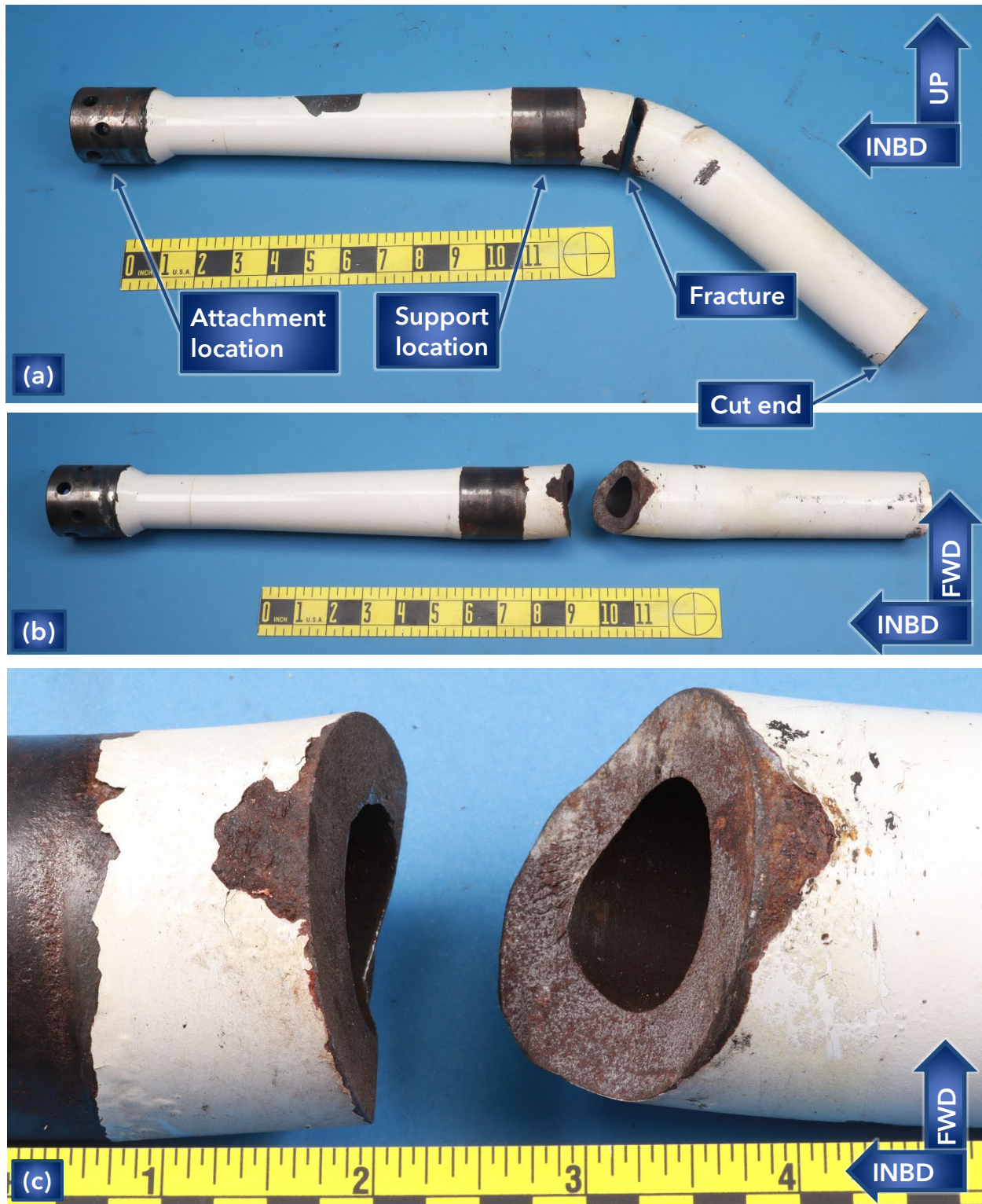
Figure 1. Overall views of the submitted main landing gear pieces as received showing (a) the aft side and (b) the lower side. (c) Closer view of the lower surface at the fracture location.
