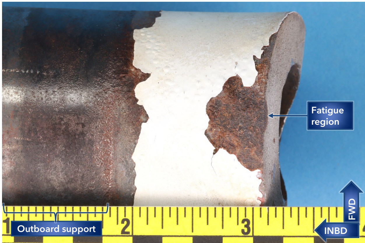
Figure 3. Closer view of the lower surface on the inboard piece of the right main landing gear after cleaning. The area showed bubbled and missing paint with substantial corrosion and pits adjacent to the fracture surface and at the outboard edge of the outboard support contact area.
