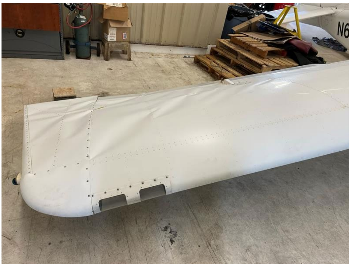
Photograph 3 - Damage to the right wing (Courtesy of the FAA)
