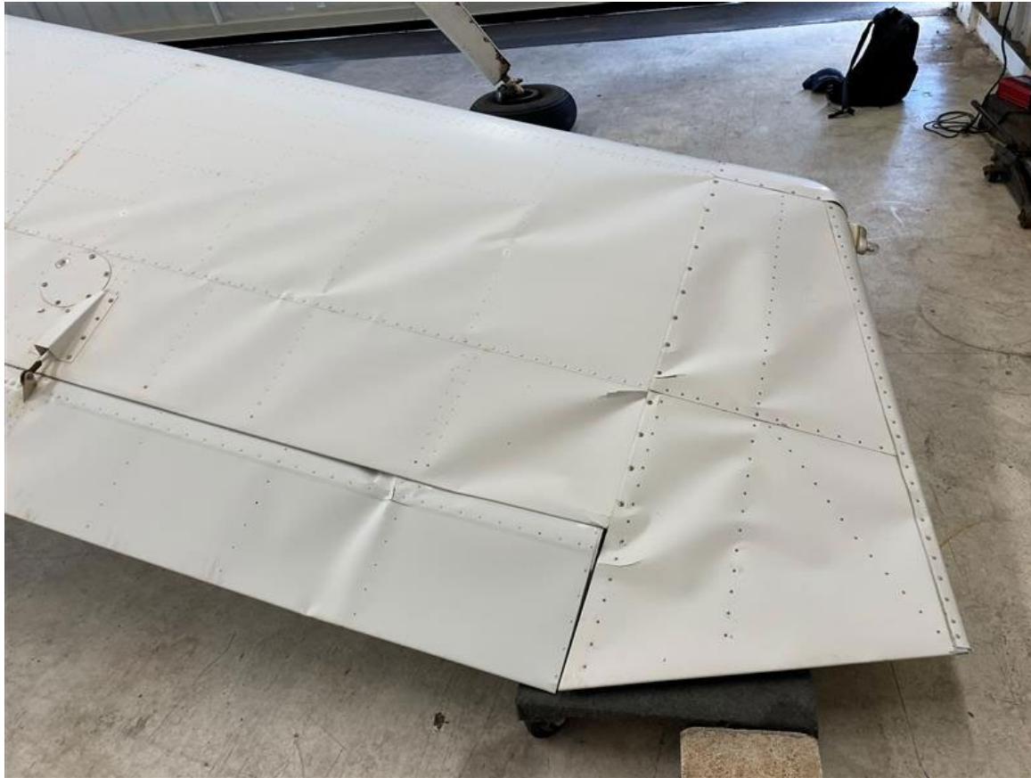
Photograph 2 - Damage to the right wing (Courtesy of the FAA)
