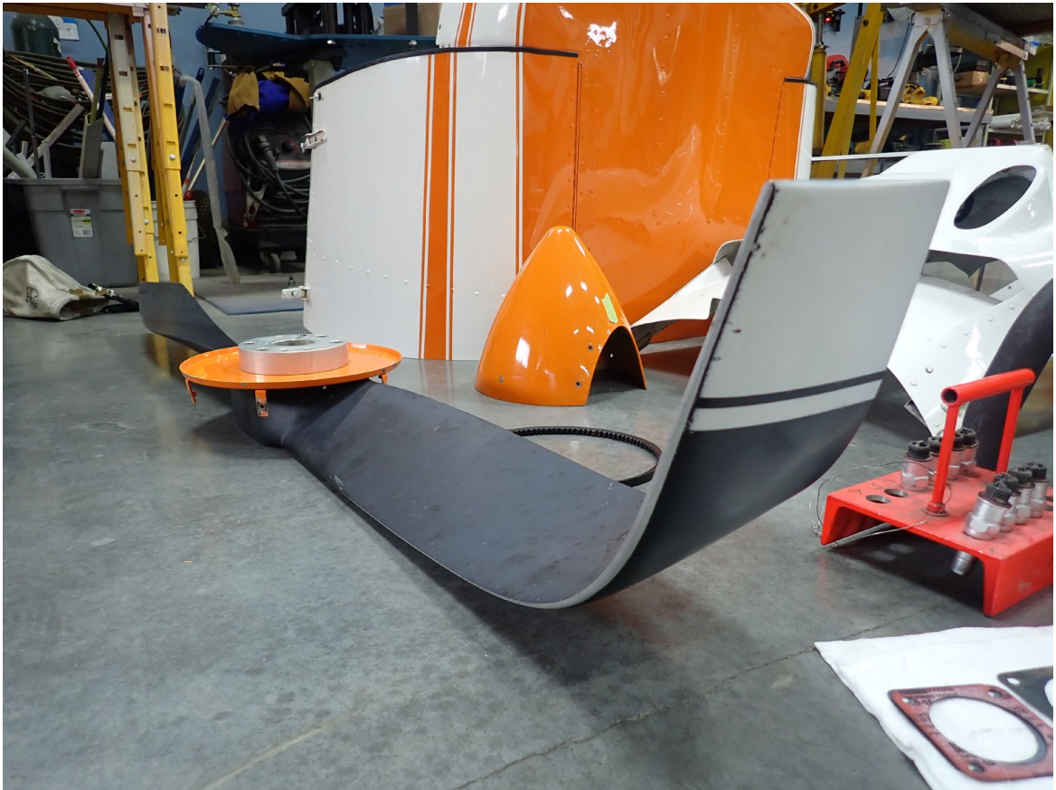
Figure 4 - Propeller with bent blade tips (NTSB Photo)
