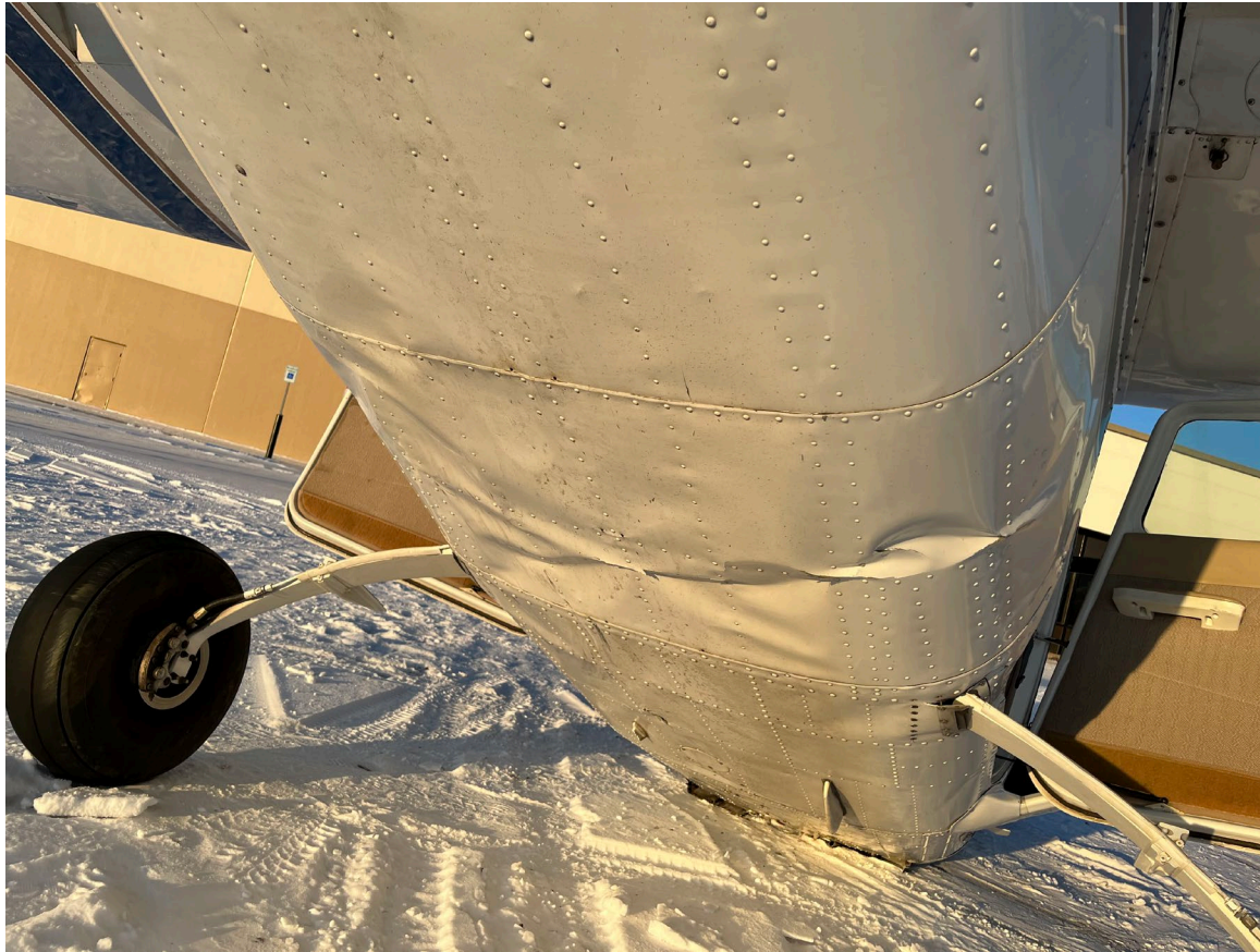
Photograph 2 - View of damage to fuselage of airplane
